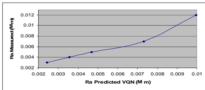
Figure (12) Scatterplot of the measured Ra and the predicted Ra by use VQN.
