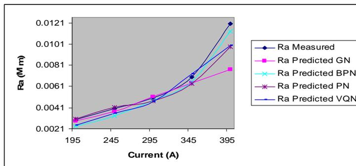
Figure (13) Effect of the current on the Ra for different network models at thickness 3mm.
