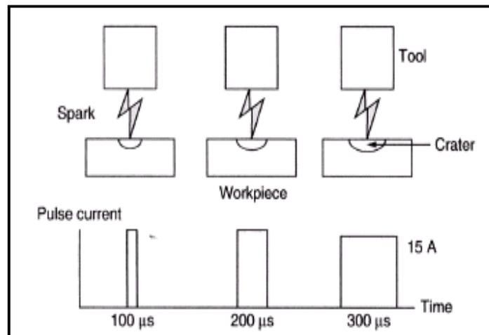
Figure (3) Effect of pulse on-time (energy) on removal rate and surface roughness [13].
