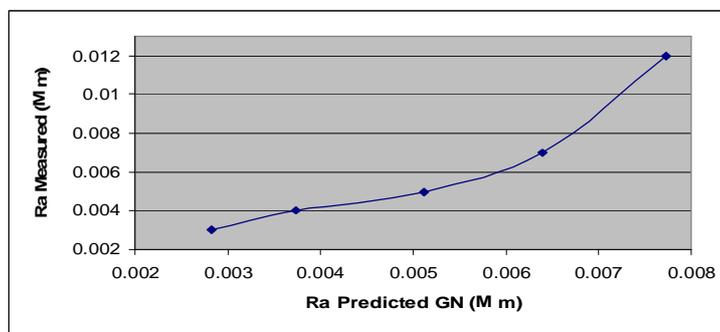
Figure (9) Scatterplot of the measured Ra and the predicted Ra by use GN.
