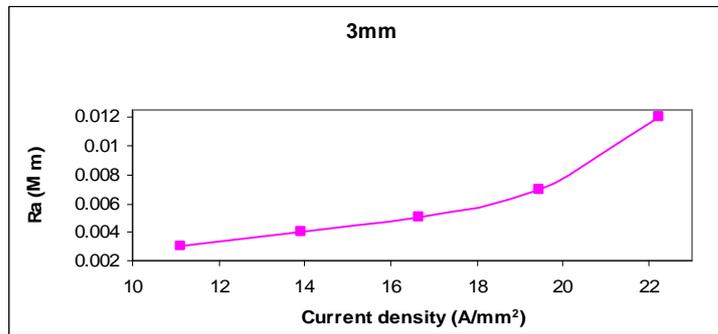
Figure (8) Effect of Ra on the current density at 3mm thickness.
