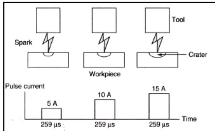
Figure (2) Effect of pulse current (energy) on removal rate and surface roughness [13].
