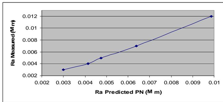
Figure (11) Scatterplot of the measured Ra and the predicted Ra by use PN.
