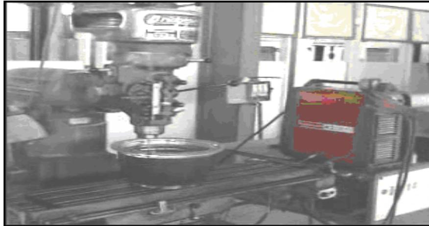
Figure (5) Universal EDM machine model.
