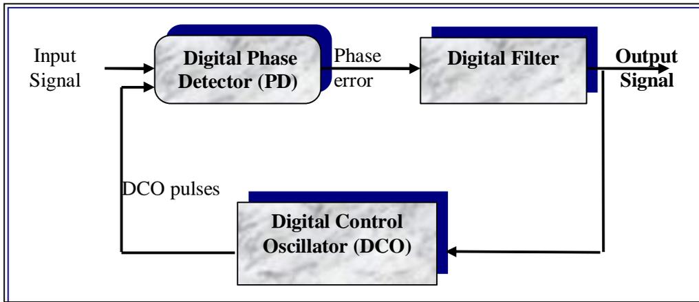
Figure (2): Block diagram of digital phase locked loop
