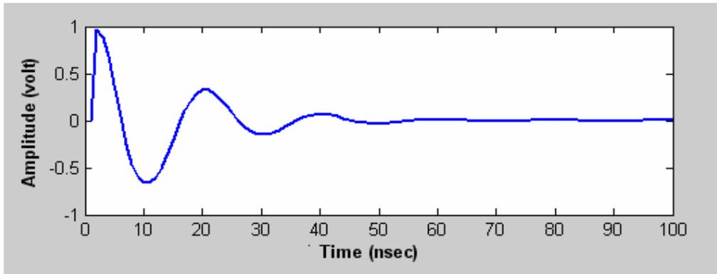
Figure (8) Output loop filter for 10 degree offset case
