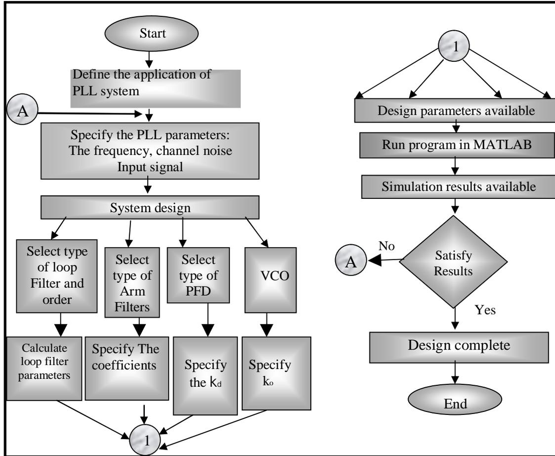
Figure (6): Flow chart of the designed system
