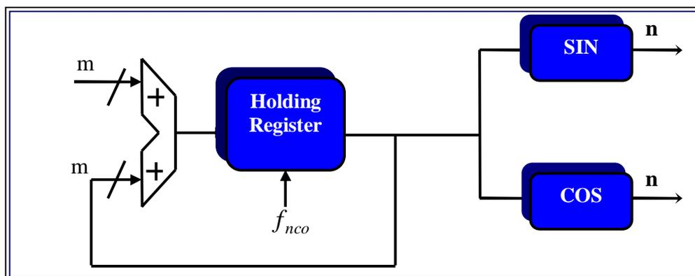
Figure (5) Direct digital frequency synthesizer (DDS)
