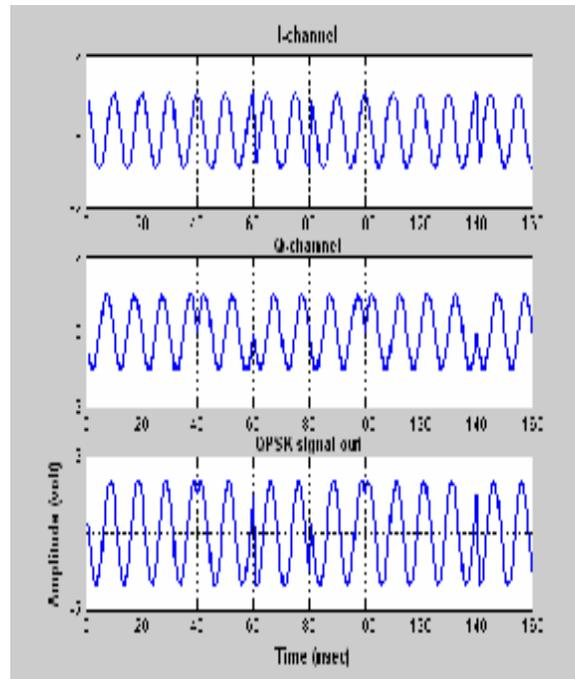
Figure (19) Simulation results of the transmitter of QPSK system
