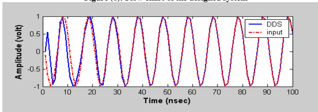
Figure (7) Input and DDS output signals for 10 degree offset case
