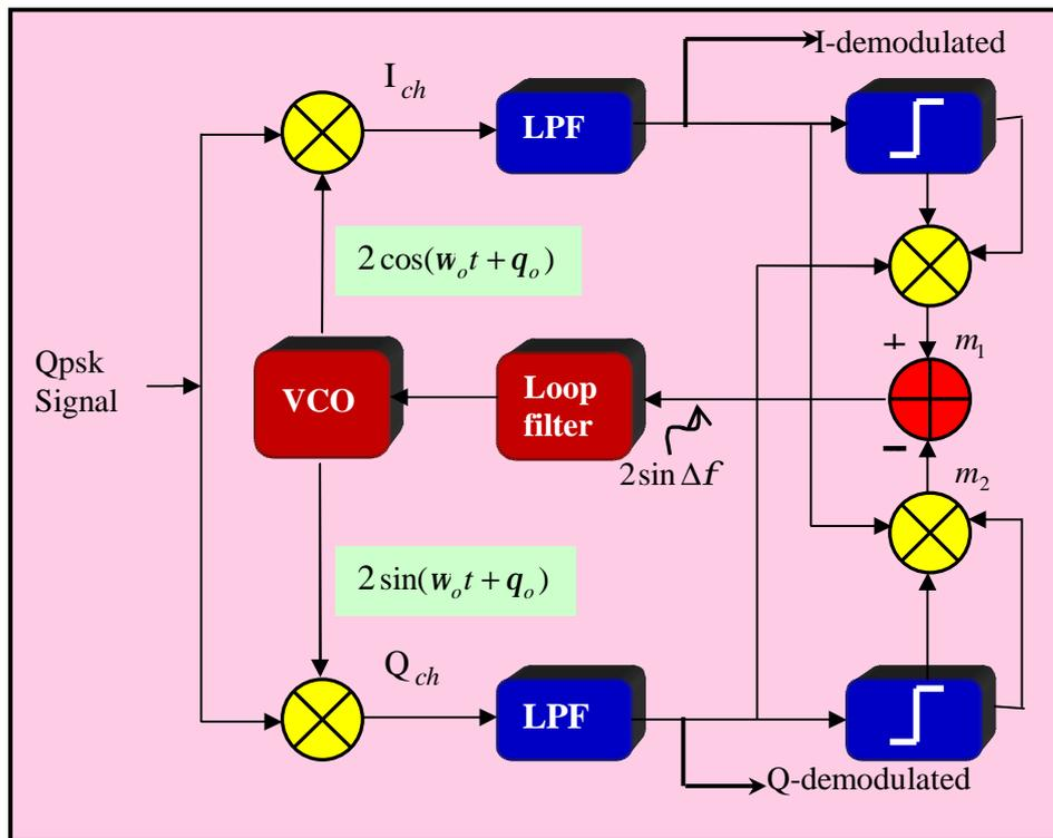
Figure (4) Costas loop for QPSK synchronizer
