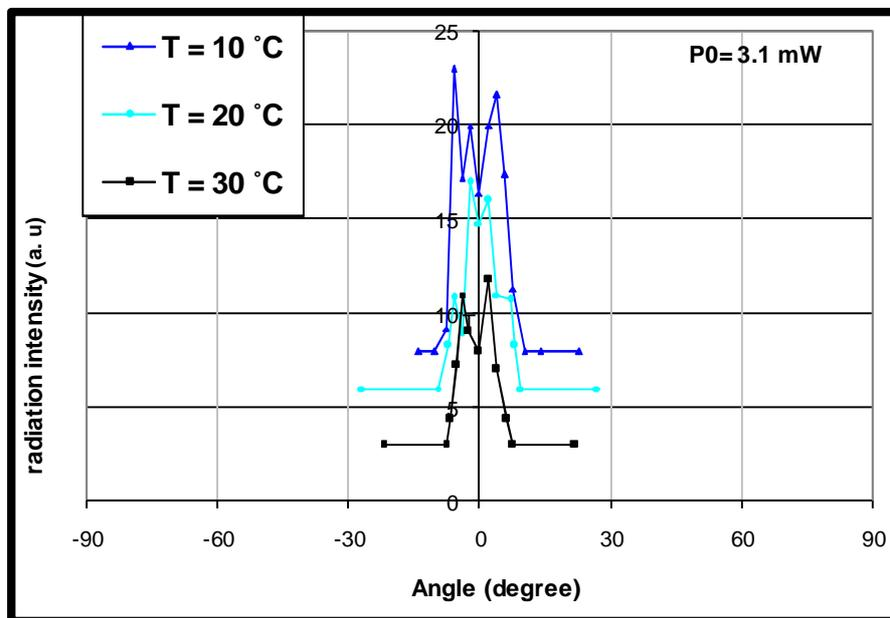
Fig (12) Temperature dependence of far pattern (parallel junction)
