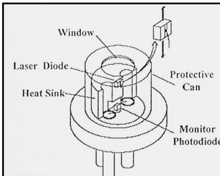
Fig (2) structure of laser diode.
