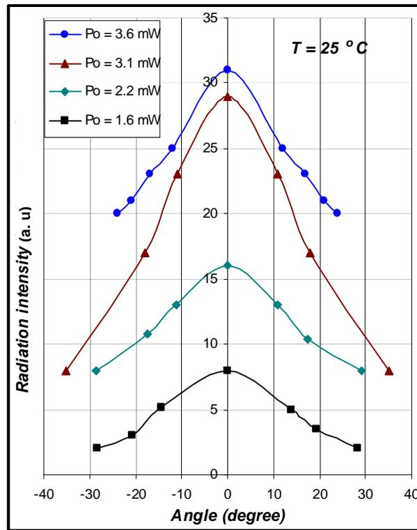
Fig(9) Power dependence of far field pattern (perpendicular to junction)
