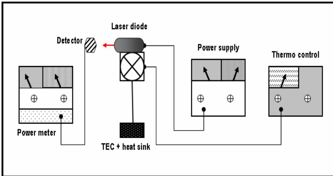
Fig (3) The Measuring of optical power as a function of forward current.
