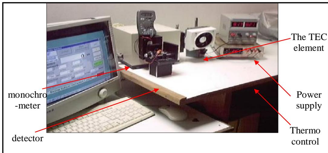
Fig (1)A photograph of the layout on the optical table
