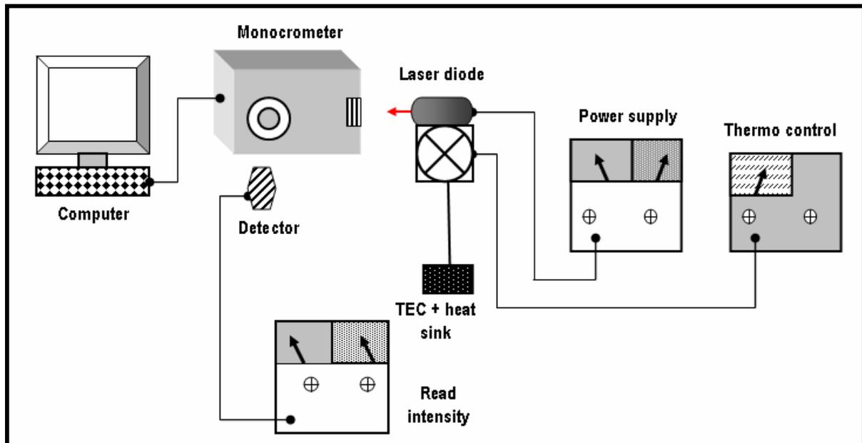
Fig (5) Measured the emission spectrum for laser diode
