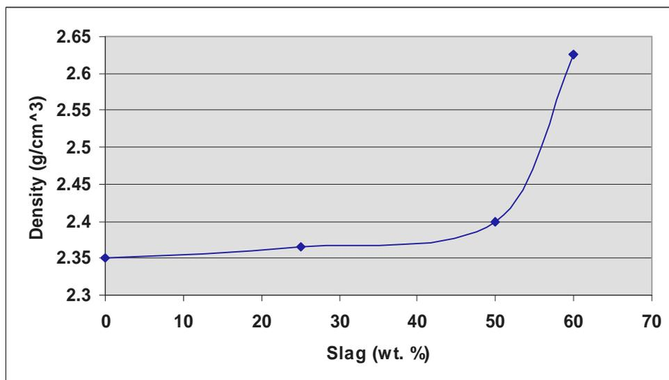
**Figure (1) The Relation Between Slag Content and Density of Cubic Samples**
