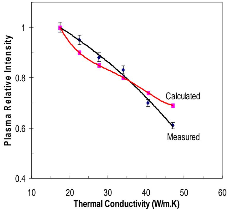
Figure (3) Variation of theoretical and experimental plasma relative intensity with Sn-Bi-Pb alloy thermal conductivity at 0.1mbar
