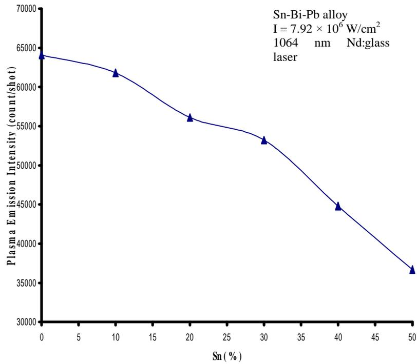
**Figure (2) Variation of plasma emission intensity of Sn-Bi-Pb alloy with Sn (%) at 0.1 mbar.**
