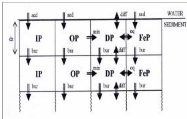
Figure (6) Illustration of the sediment phosphorus model.
