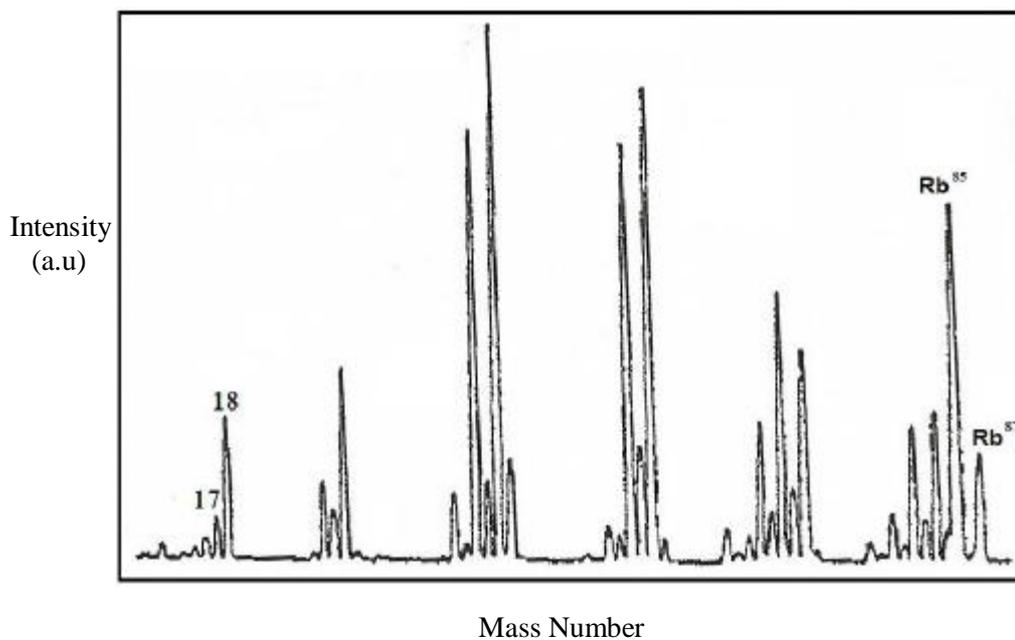
Figure (3b) Effusive atomic beam spectrum at  $T=850$  °C,
