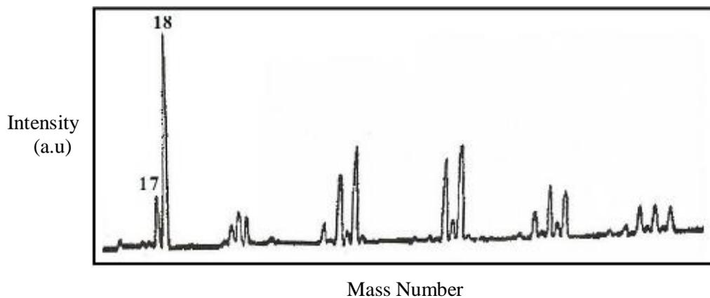
Figure (3a) Background Spectrum at a chamber pressure of  $10^{-7}$  mbar
