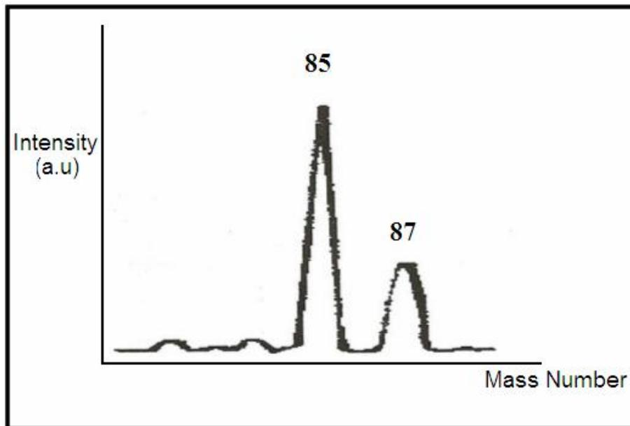
Figure (4) Rubidium isotopes ( $Rb^{85}$ ,  $Rb^{87}$ ) at  $T= 850$  °C using quadruple ion source ( $I=20 \times 10^{-11}$  Amp.)
