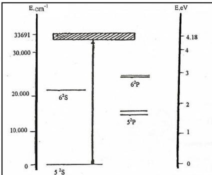
Figure (1) Energy level Scheme for Rb Atom [8]
