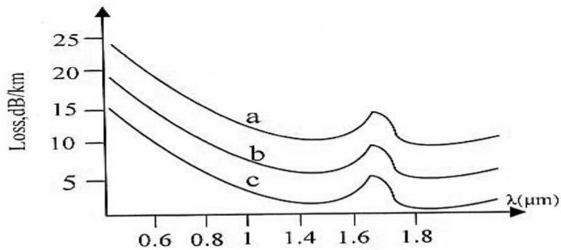
Fig. dependence of loss on fiber drawing temperature (Exp.step-index fiber with  $\Delta n_1=0.013$ :) (a),(b),(c) different temperature.
