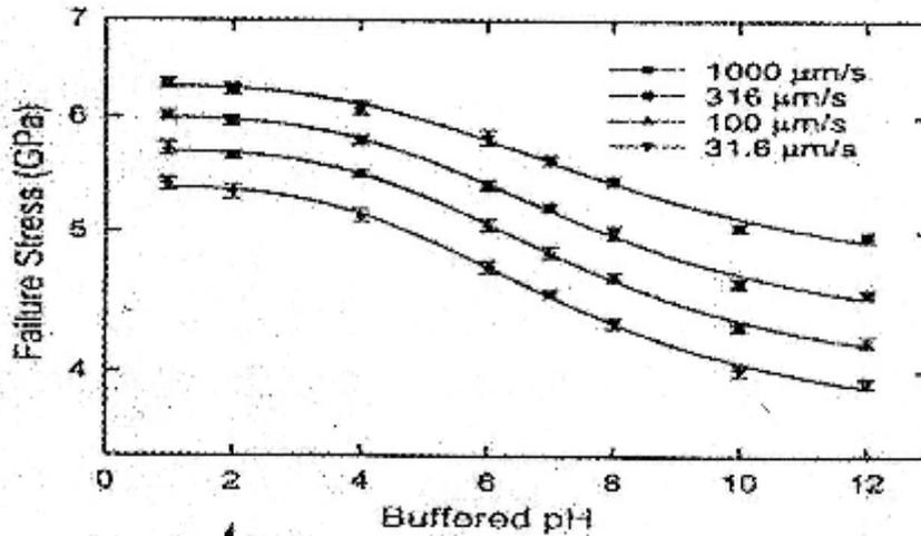
Figure (1) Strength as a function of pH at four different faceplate speeds for measurements made in two-point bending
