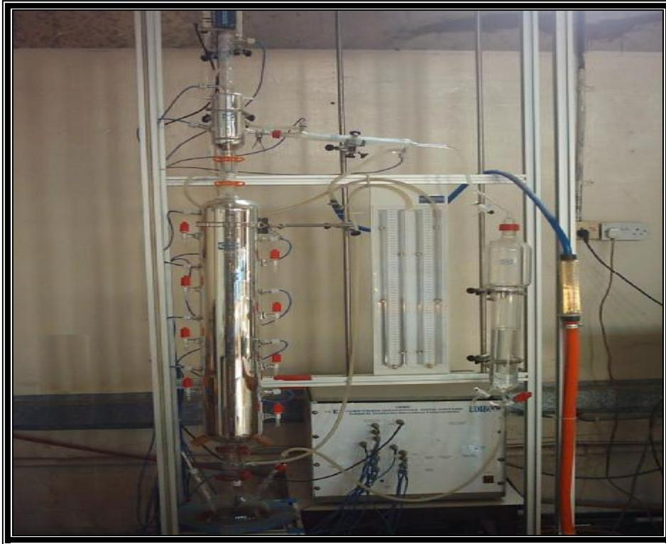
Figure (1): Photograph for The Experimental Rig of Batch Distillation Column.
