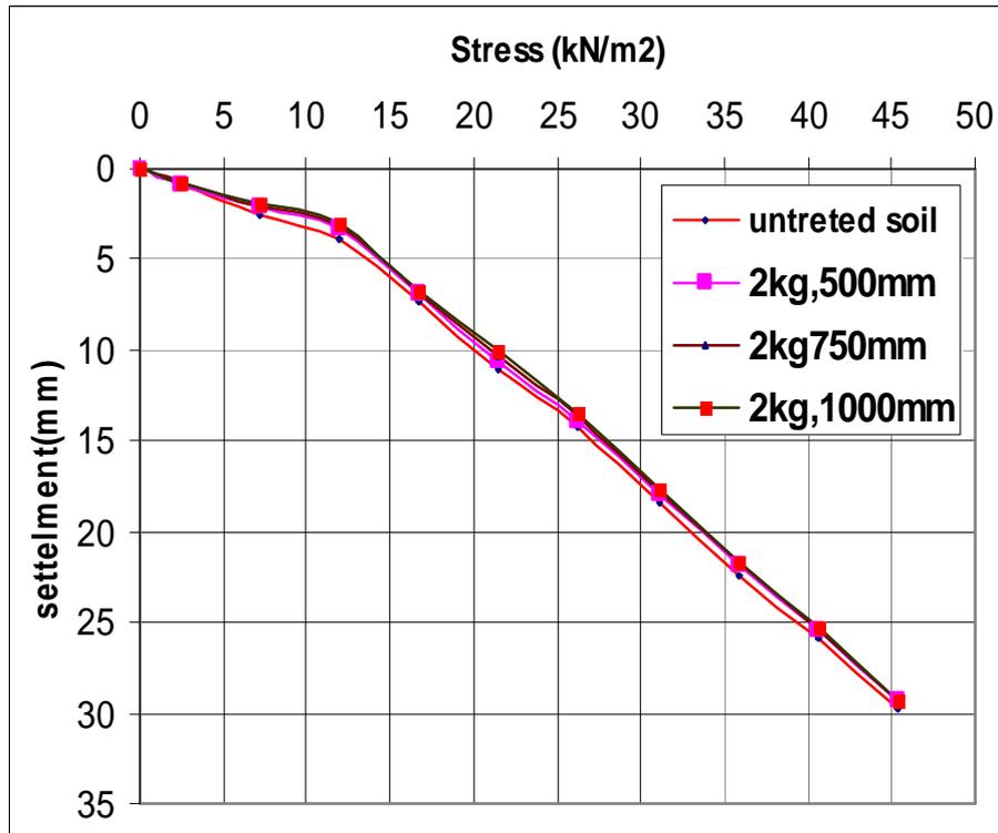
Figure (7) Stress-settlement curve for untreated and treated soil using dynamic compaction(weight 2kg, heights of drop 500,750,1000mm).
