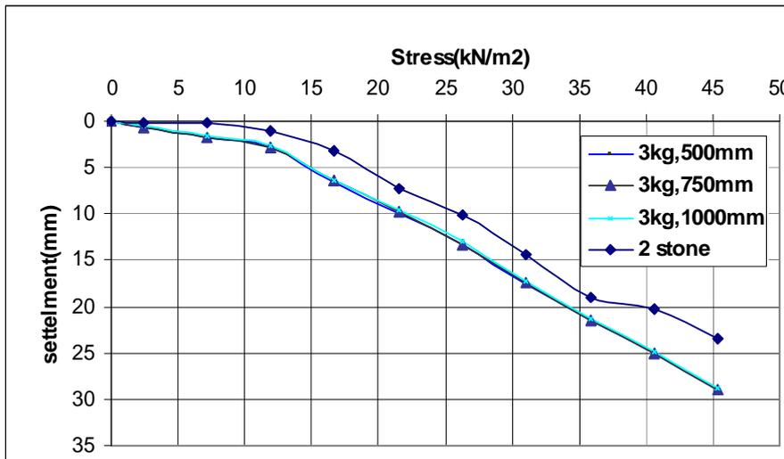
Figure (15) Stress-settlement curve for treated soil using 2 stone columns and dynamic compaction (weight 3kg , heights of drop 500,750,1000mm).
