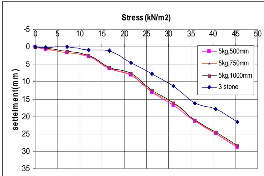
Figure (16) Stress-settlement curve for treated soil using 3 stone columns and dynamic compaction (weight 5kg , heights of drop 500,750,1000mm).
