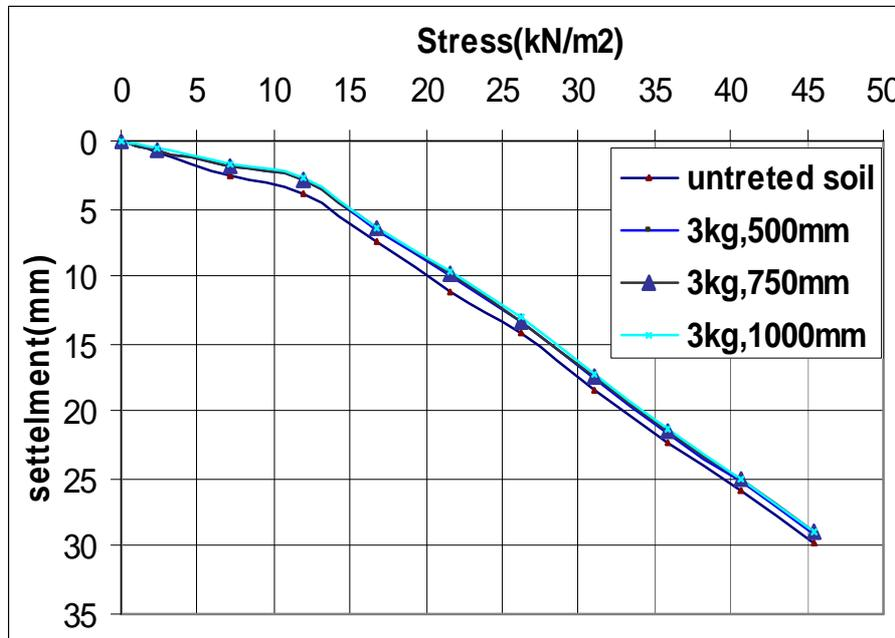
Figure (8) Stress-settlement curve for untreated and treated soils using dynamic compaction (weight 3kg, heights of drop 500, 750, 1000mm).
