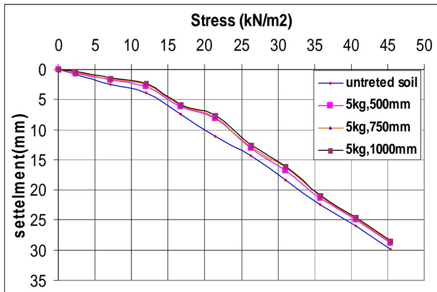
Figure (9) Stress-settlement curve for untreated and treated soils using dynamic compaction (weight 5kg, heights of drop 500, 750, 1000mm).
