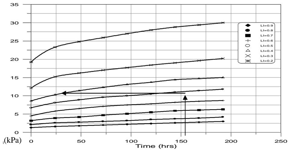
Figure (5) Variation in untrained shear strength versus time for remolded clay.
