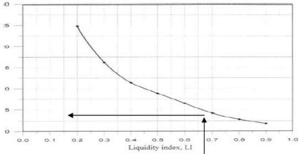
Figure (4) . Variation of undrained shear strength versus liquidity index for remolded clay after 48 hrs.
