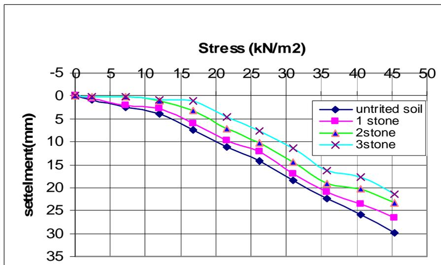
Figure (13) Stress-settlement curve for untreated and treated soils using stone columns (1 ,2 and 3 stone columns).
