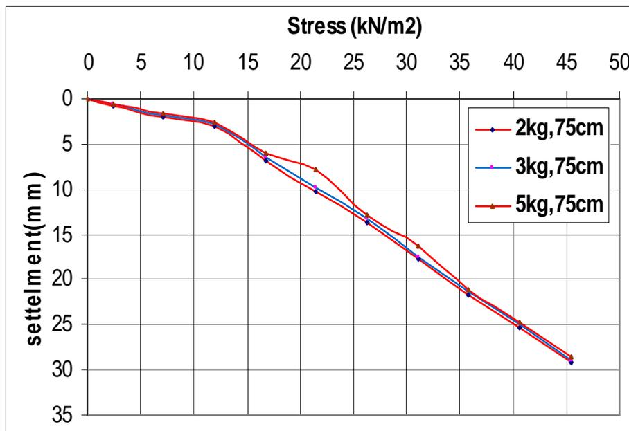
Figure (11) Stress-settlement curve for untreated and treated soils using dynamic compaction (weights 2, 3, 5 kg heights of drop 750 mm).
