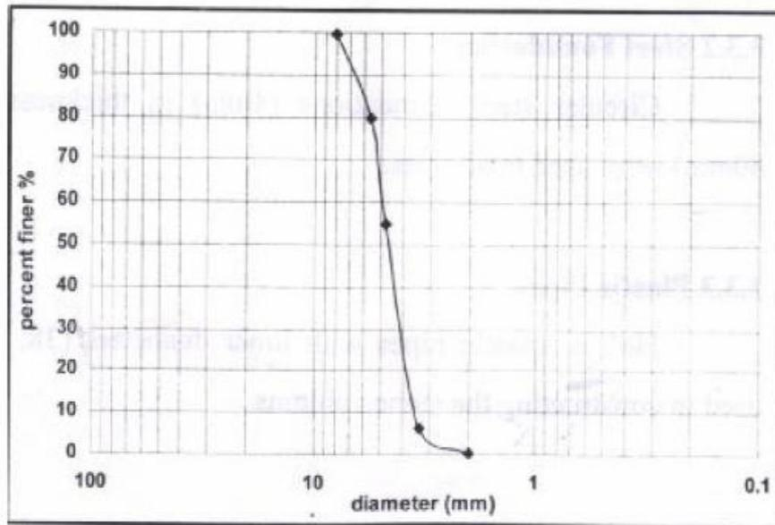
Figure (2) Grain size distribution of crushed stone used.
