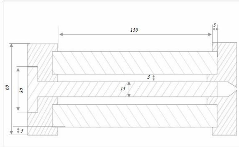
Figure 1 : Cross section view of the steel mould dimension are in mm.
