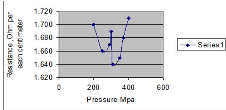
Figure (3) Effect of increasing pressure (20-40) Mpa on the measured resistance
