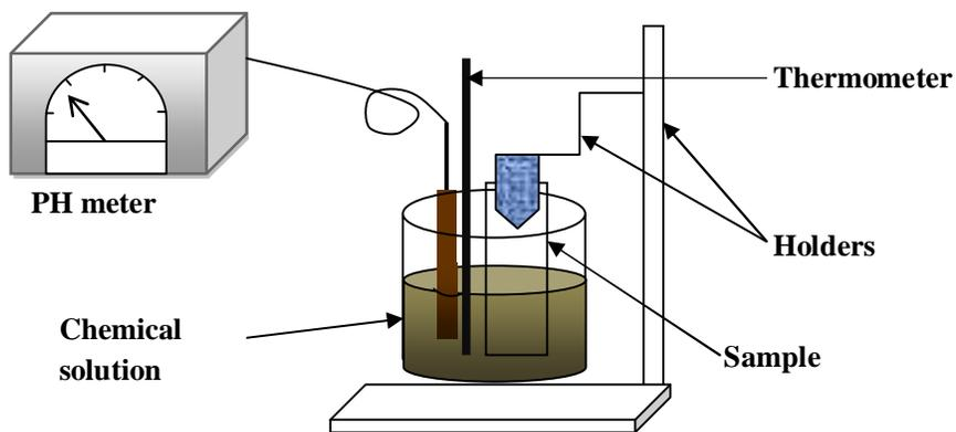
Figure (1) show the setup of deposition system
