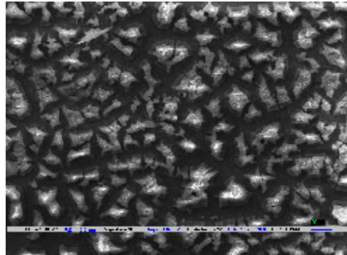
Figure (3) SEM micrograph of the surface of porous silicon layer prepared by photoelectrochemical etching.
