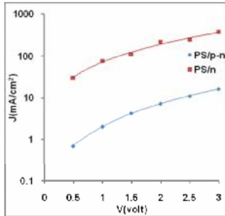
Figure (2) I-V characteristics at different substrate.
