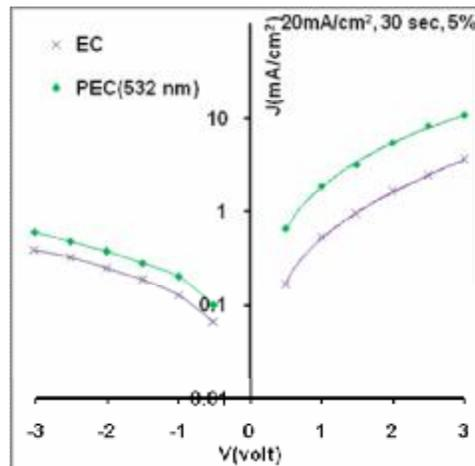
**Figure (1) Dark, forward bias and reverse bias I-V characteristics of nanostructured solar cell.**
