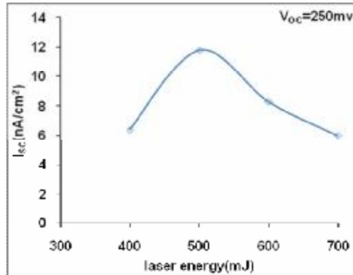
Figure (6) Effect laser energy on short circuit current of solar cell.
