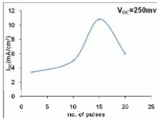
Figure (7) Effect no. of laser pulses on  $I_{SC}$  at  $V_{OC} = 250\text{mv}$ .
