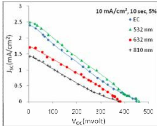
Figure (5) Effect of wavelength on  $I_{SC}$ - $V_{OC}$  characteristics of solar cell.
