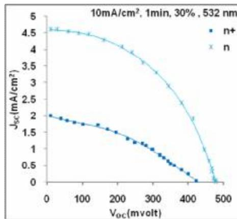
Figure (4) Effect of substrate resistivity on characteristics of nanostructure solar cell.
