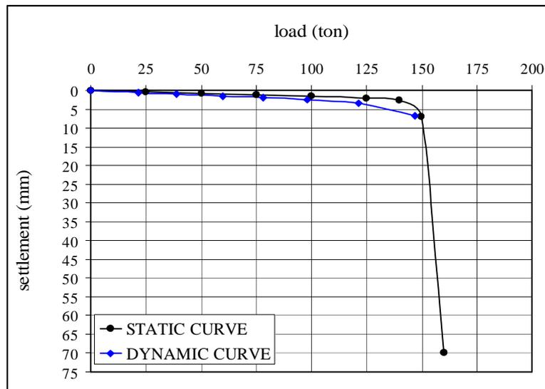
**Figure (1) Comparison between actual (Static Load Test) and simulated (PDA/CAPWAP Dynamic Test) results (P76- S3)**
