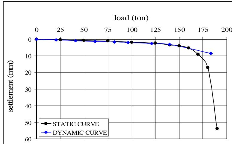
Figure (2) Comparison between actual (Static Load Test) and simulated (PDA/CAPWAP Dynamic Test) results (P54- S3).
