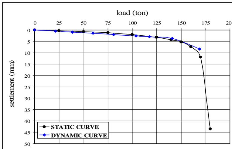
Figure (3) Comparison between actual (Static Load Test) and simulated (PDA/CAPWAP Dynamic Test) results (P72- S3).
