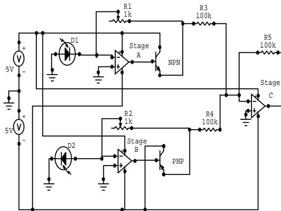
Figure (3) Electronic circuit of laser power comparator.
