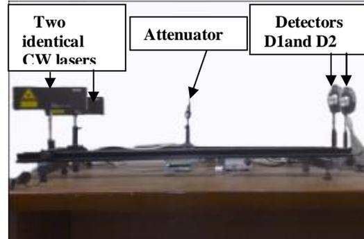
Figure (4) Optical arrangement of the laser power comparator.
