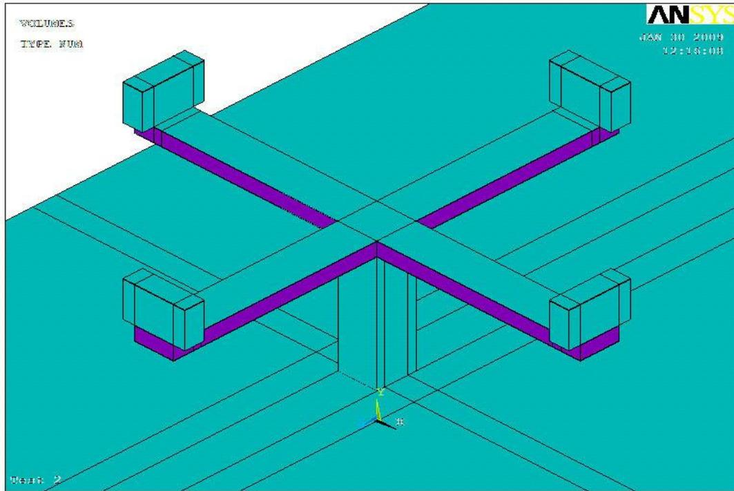
Figure (5): Four arms damper configuration
