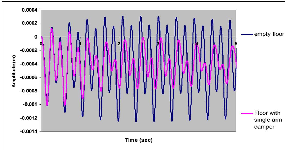
Figure (11): Transient response amplitude of the concrete floor with and without the single arm viscoelastic damper attached.
