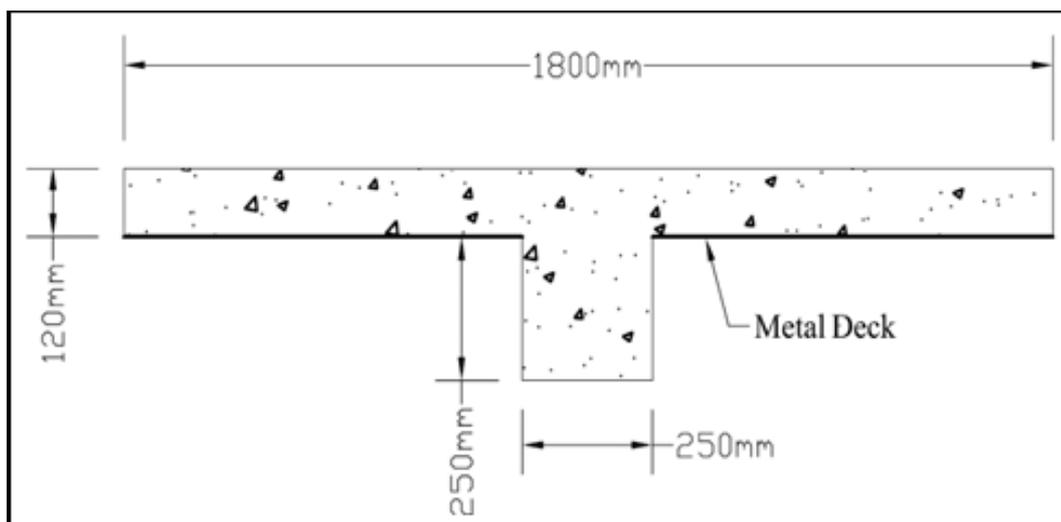
Figure (6): Concrete floor cross sectional area
