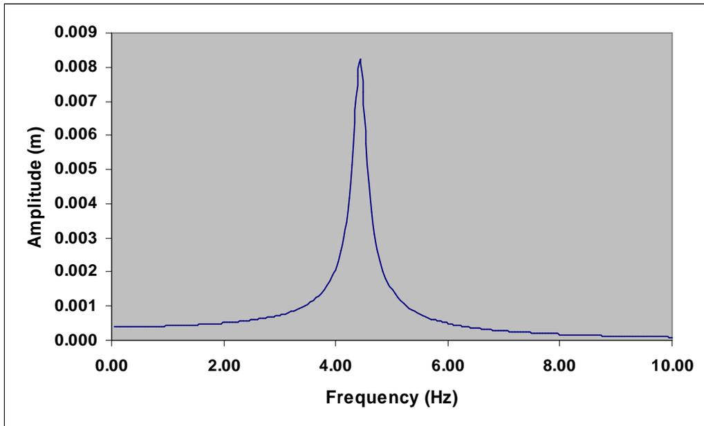
Figure (7): Fundamental frequency of floor
