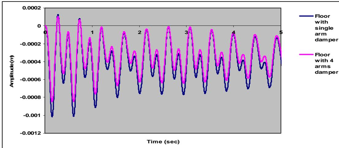
Figure (13): Comparison between transient response amplitudes of the concrete floor with the single arm or the four arms viscoelastic damper
