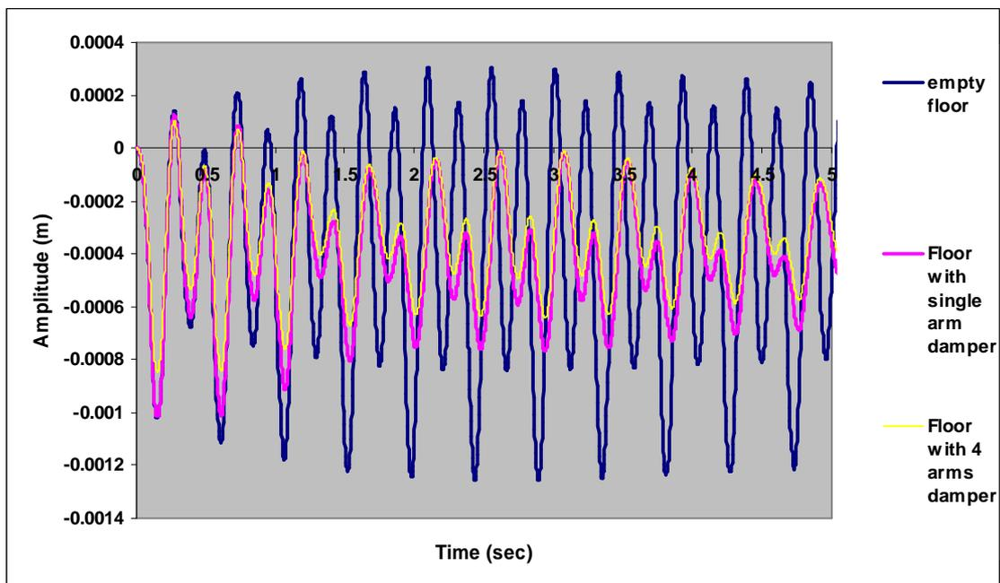
Figure (14): Comparison between the effectiveness of the single arm and the four arms viscoelastic dampers in suppressing floor vibration.
