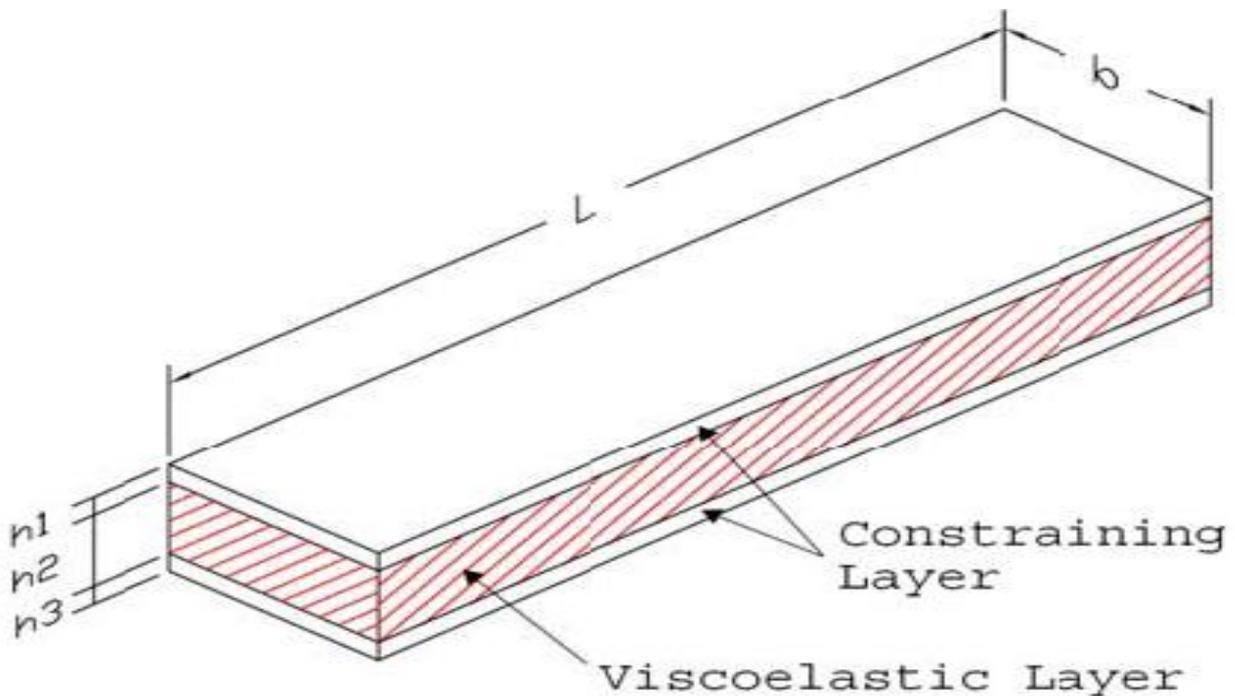
Figure (2): Constrained layers configuration [10]
