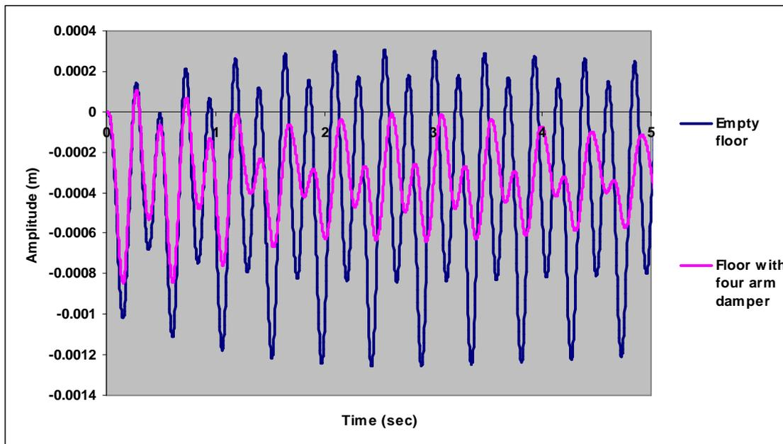
Figure (12): Transient response amplitude of the concrete floor with and without the four arms viscoelastic damper attached.
