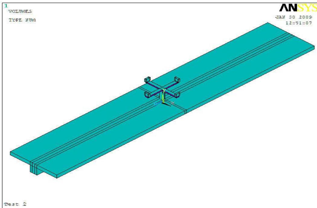
Figure (10): Floor-Four arms damper coupled system
