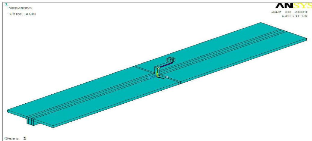
Figure (9): Floor-Single arm damper coupled system
