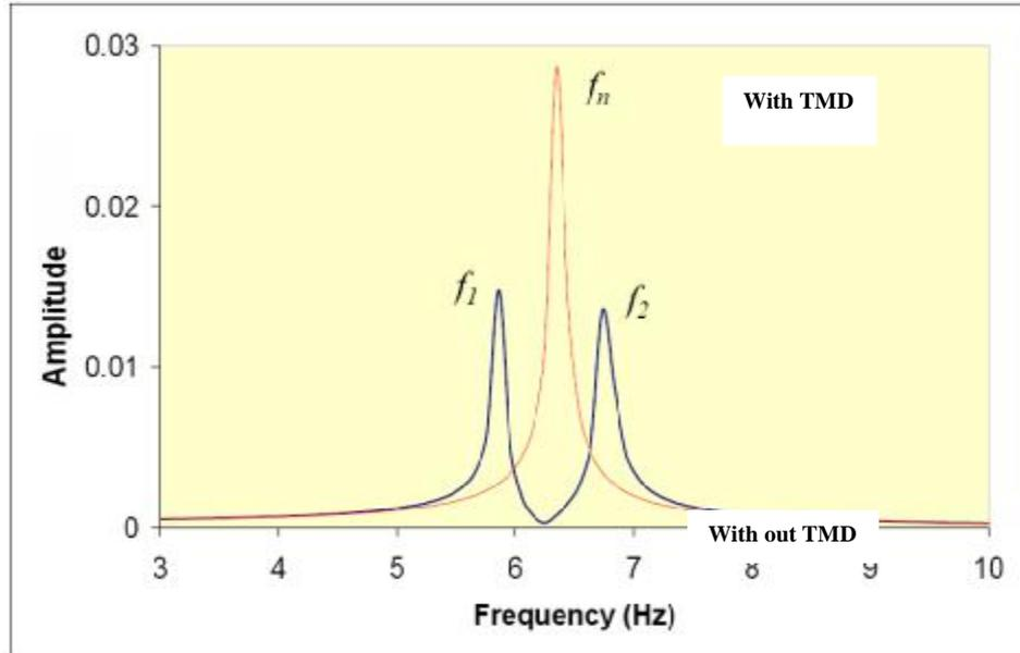
Figure (1): An example showing the effects of attaching a TMD to a primary system [10]
