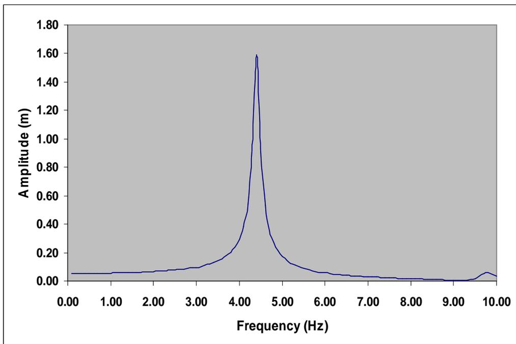
Figure (8): Fundamental frequency of damper
