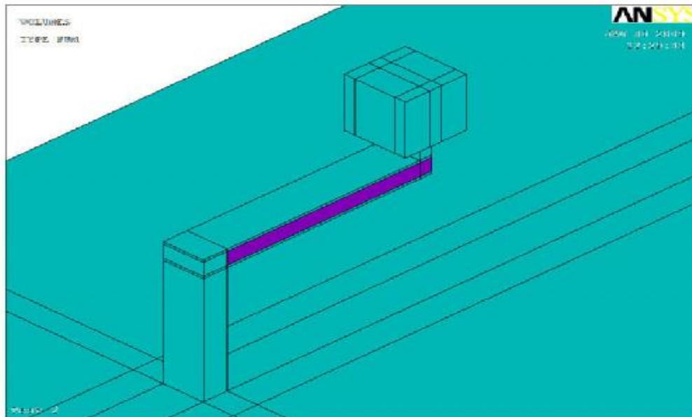
Figure (4): Single arm damper configuration
