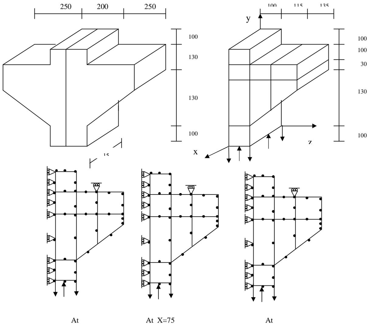
Fig.(5). Finite element mesh and conditions in Muhammad's corbels.
