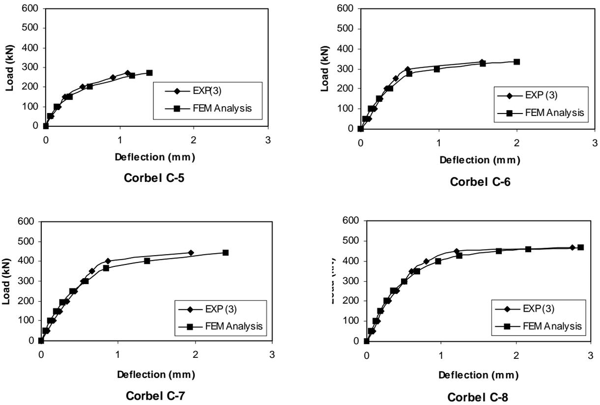
Fig.(6).Muhammads corbels, analytical and experimental load- deflection curves.
