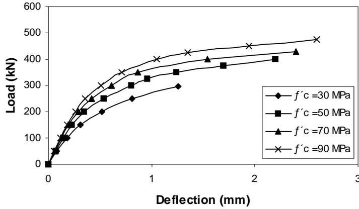
Fig.(8) Effect of increasing the grades of concrete on the load - deflection behavior for corbel C-7
