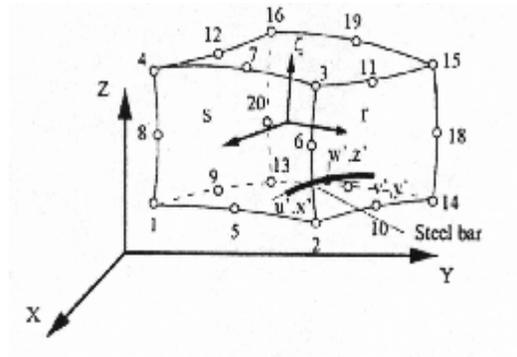
Fig. (1) The twenty-node brick element.
