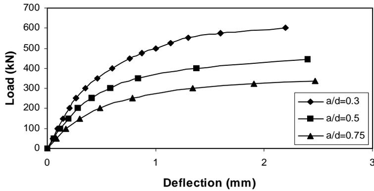
Fig. (10) Influence of shear span-depth ( $a/d$ ) ratio on load-deflection curve for corbel C-7
