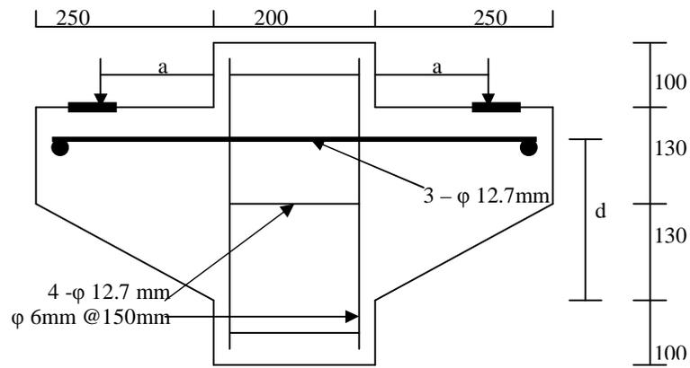
Fig.(4).Dimensions and reinforcement details of Muhammad's corbels (3)
