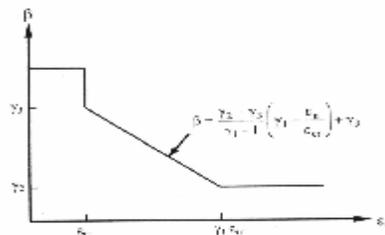
Fig. (3) Shear retention model for cracked concrete.
