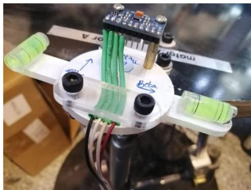
FIG. 11. MPU6050 SENSOR.
