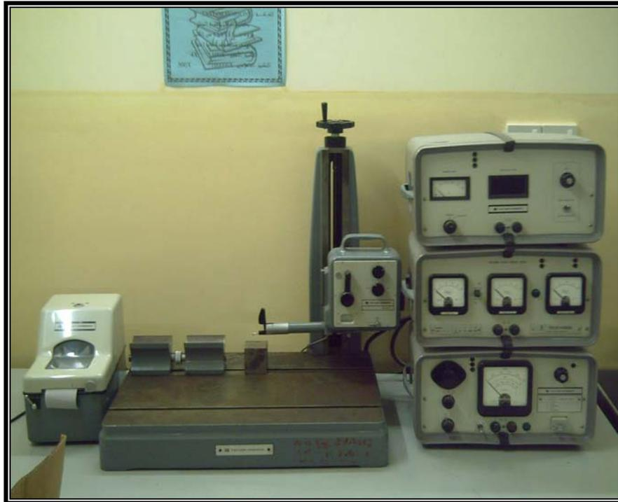
**Fig. (3): Roughness apparatus measurement**
