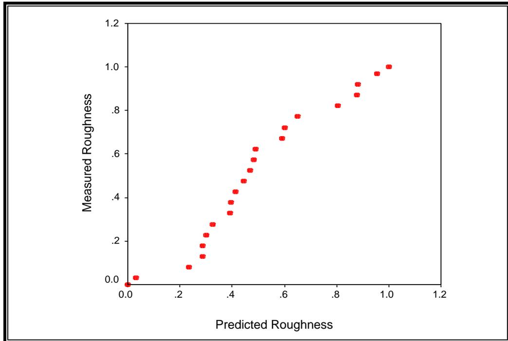
Fig. (4): Scatterplot of the Measured Ra and the Predicted Ra of the Multiple Regression Prediction Model for 4-Flute end mill using (SPSS)
