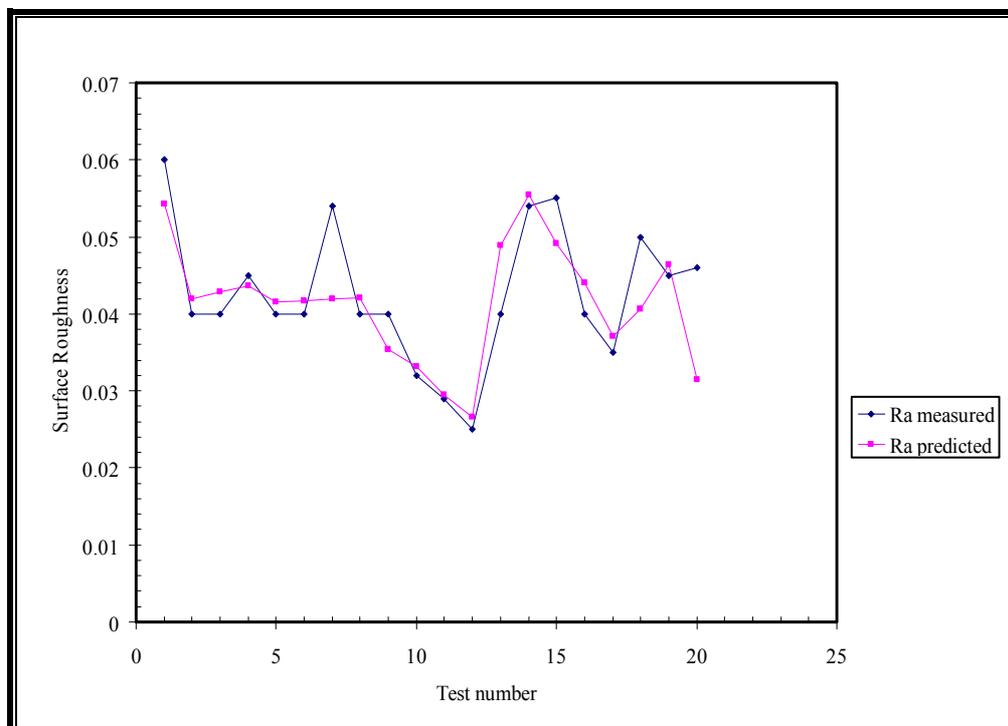
Fig. (5): The diagram of the measured and predicted surface roughness for the experimental data using the commercial statistical package (SPSS) for 4-Flute end mill
