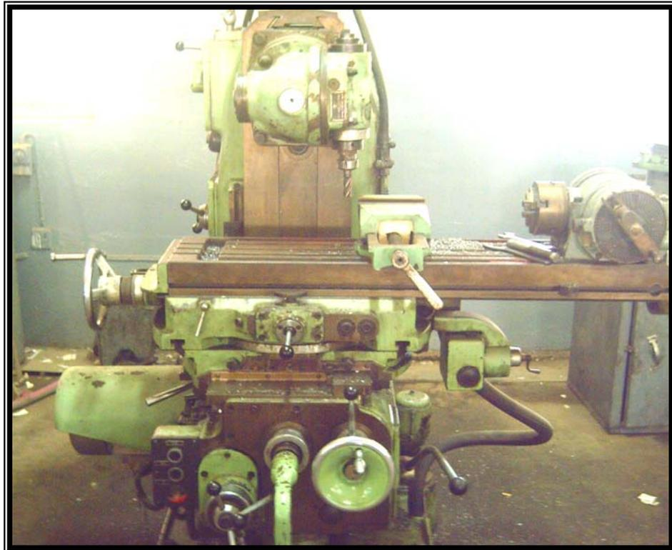
**Fig. (1): Universal milling machine model (6H81)**
