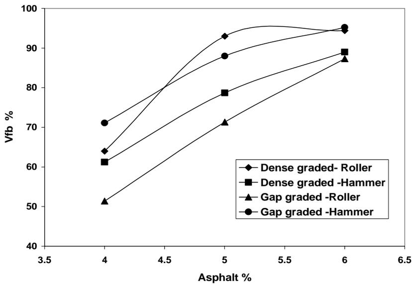
FIGURE 4 Voids filled with bitumen for Asphalt Concrete mixes
