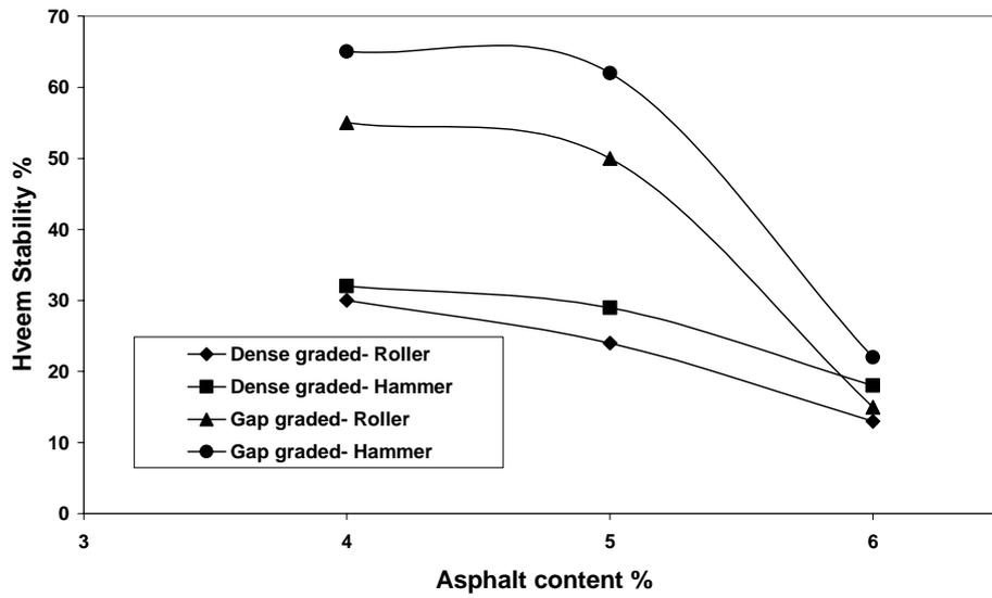
FIGURE 7 Hveem Stability of Asphalt Concrete
