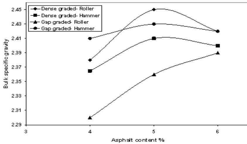
**FIGURE 5 Bulk specific gravity of Asphalt Concrete mixes**
