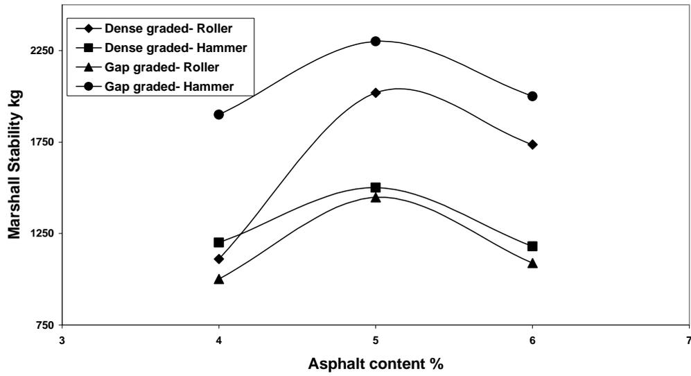
FIGURE 1 Marshall stability of Asphalt Concrete
