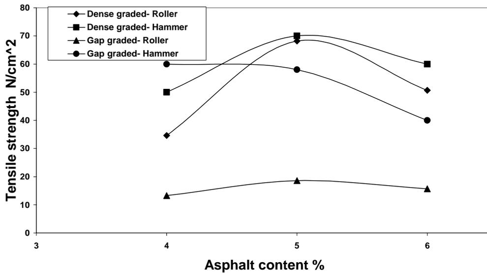
FIGURE 8 Tensile strength of Asphalt Concrete
