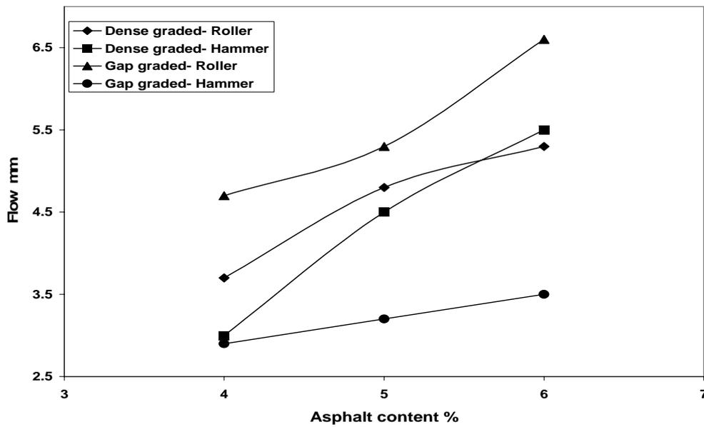
FIGURE 2 Marshall Flow of Asphalt Concrete mixes
