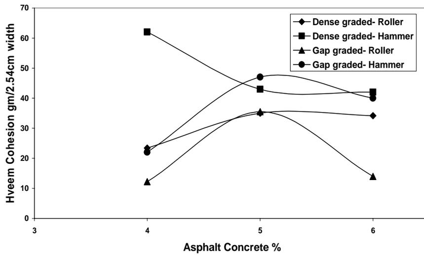
**FIGURE 6 Hveem cohesion of Asphalt Concrete**
