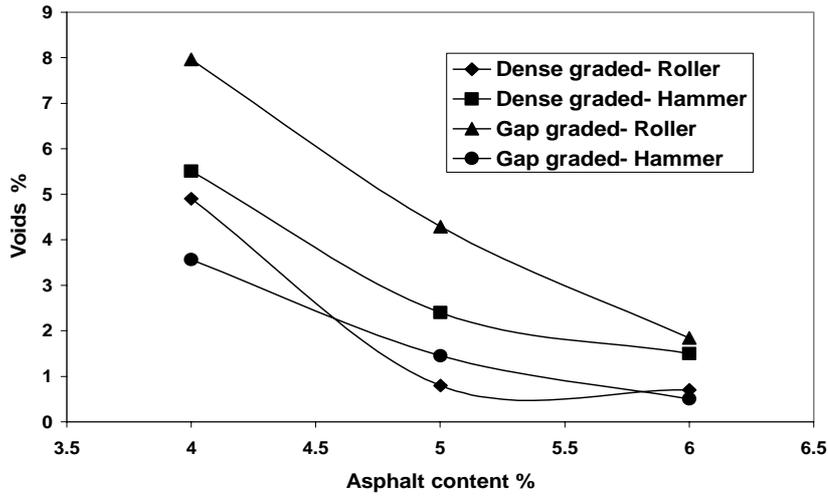
FIGURE 3 Voids % in the Asphalt concrete mixes
