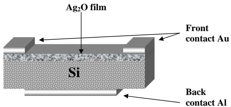
**Fig.2** Cross-section view of the final HJ.
