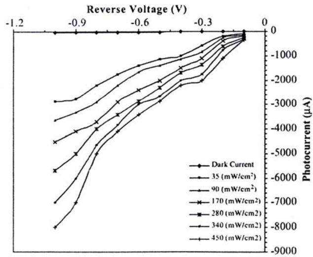
Fig. 7. I-V characteristics under illumination conditions.
