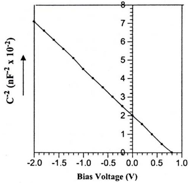
Fig.9 C<sup>-2</sup> -V of Ag<sub>2</sub>O/Si H.J
