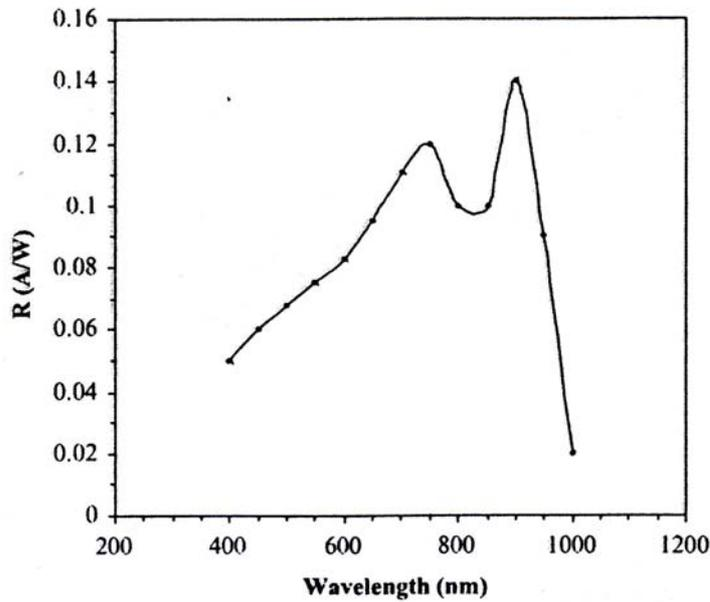
Fig.(10) show responsivity as function of the wavelength
