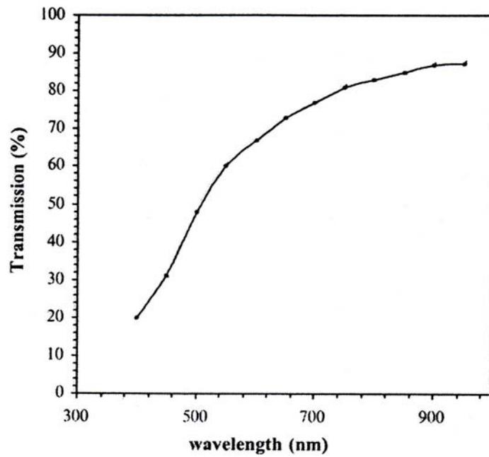
Fig.4 Transmission spectrum of Ag<sub>2</sub>O film.
