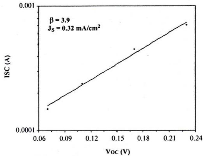
Fig. 8 Isc-Voc curve under different illumination condition
