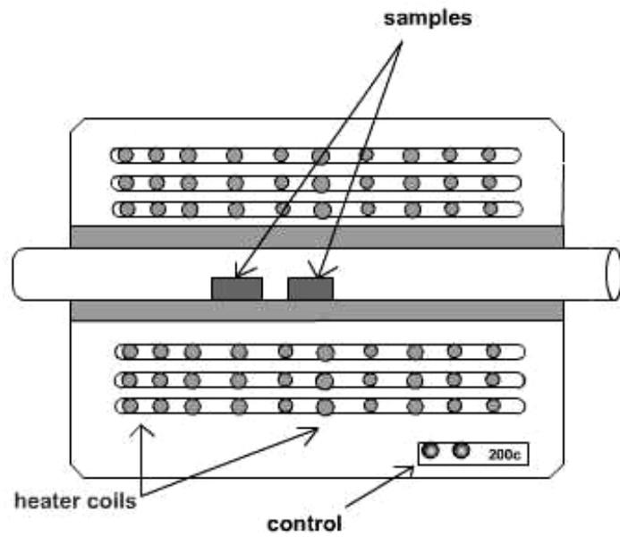
**Fig.1** Schematic diagram of furnace system.
