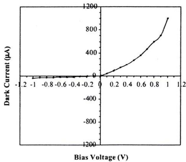
**Fig. 6 I-V characteristics of  $\text{Ag}_2\text{O}/\text{p-Si}$  isotype HJ.**
