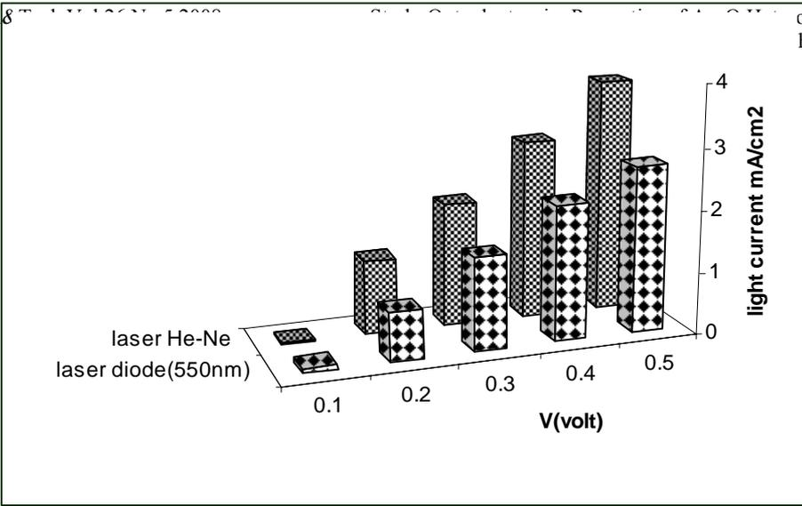
**Fig. (11) light current characteristics of Ag<sub>2</sub>O-on-Si heterojunction using 1mW He-Ne laser and 1mW diode laser(550nm).**
