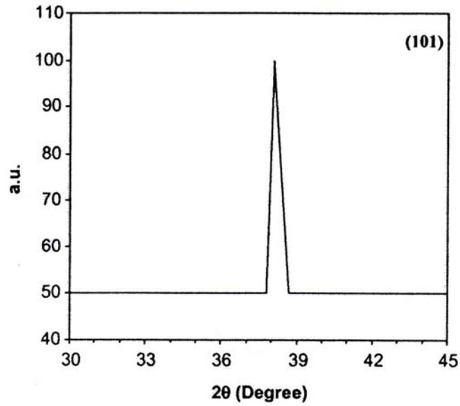
Fig.3 XRD pattern of Ag<sub>2</sub>O thin film.
