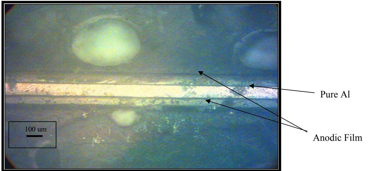
**Figure (8) Optical microscope section showing anodic film thickness of pure aluminum under ideal conditions .**
