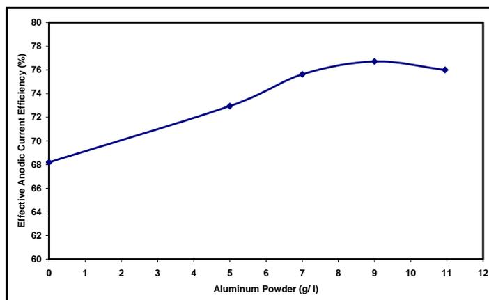
Figure (4) the effect of adding aluminum powder to anodizing solution at ideal conditions for pure aluminum on effective anodic current efficiency.
