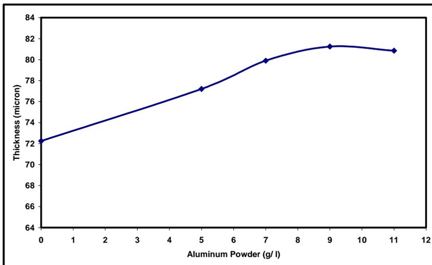
Figure (2) the effect of adding aluminum powder to anodizing solution at ideal conditions for pure aluminum on film thickness.
