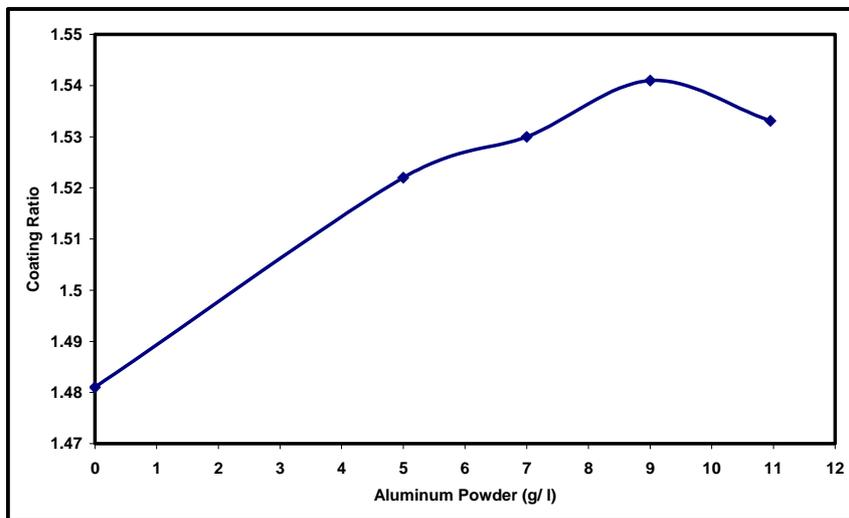
Figure (3) the effect of adding aluminum powder to anodizing solution at ideal conditions for pure aluminum on coating ratio.
