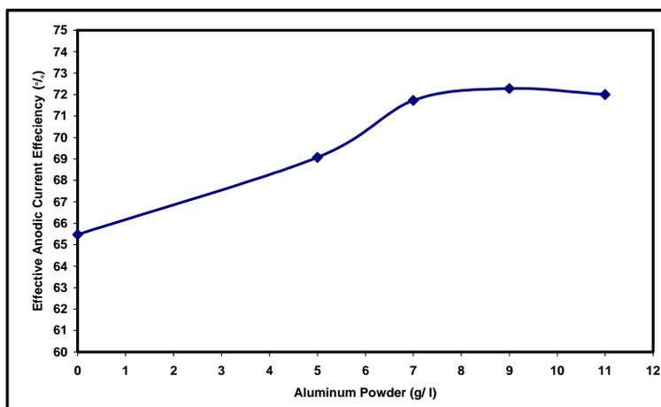
Figure (7) the effect of adding aluminum powder to ideal conditions for aluminum alloy(6063) on effective anodic current efficiency.
