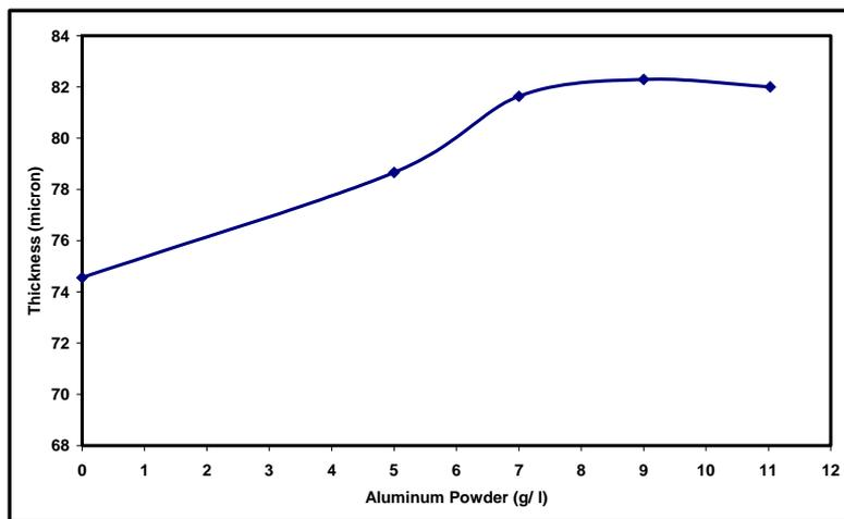
Figure(5) The effect on film thickness of adding aluminum powder to anodizing solution at ideal conditions for aluminum alloy (6063).
