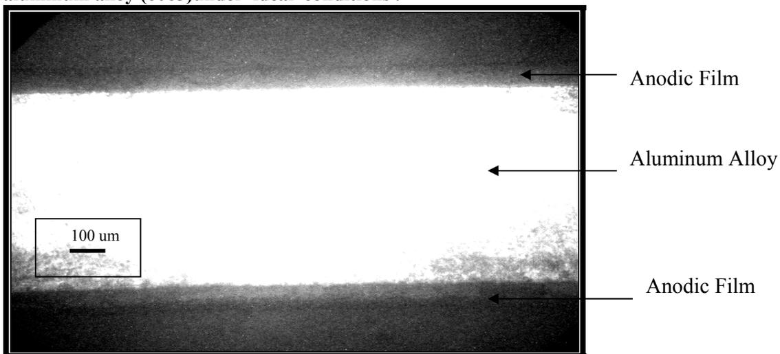
**Figure (11) Optical microscope section showing anodic film thickness of aluminum alloy (6063) under ideal conditions with 9g/l aluminum powder.**
