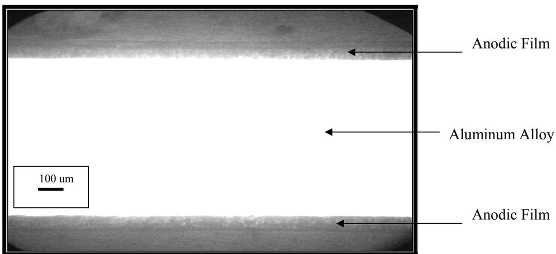
**Figure (10) Optical microscope section showing anodic film thickness of aluminum alloy (6063) under ideal conditions .**
