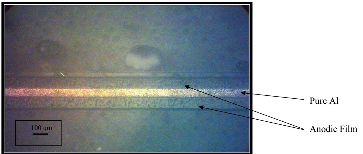
**Figure (9) Optical microscope section showing anodic film thickness of pure aluminum under ideal conditions with 9g/l aluminum powder.**
