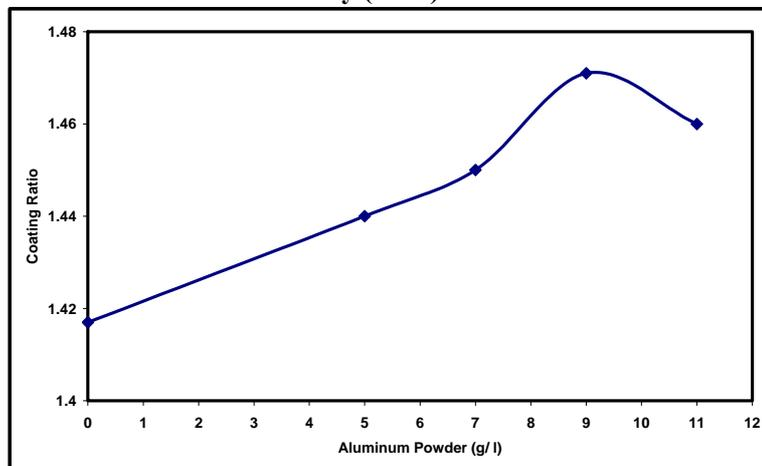
Figure (6) the effect of adding aluminum powder to anodizing solution at ideal conditions for aluminum alloy (6063) on coating ratio.
