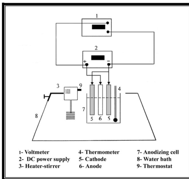
**Figure (1) schematic diagram for the whole assembly of the anodizing apparatus.**
