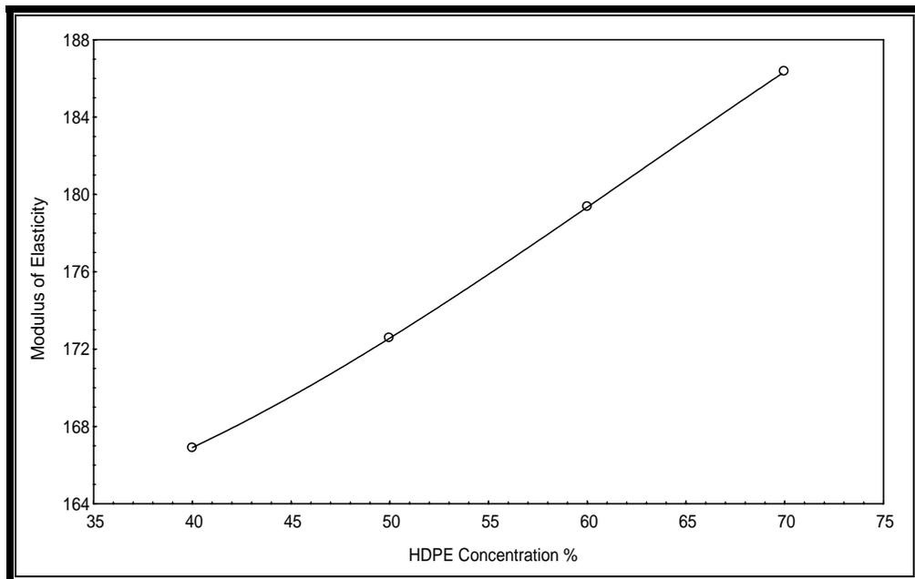
**Fig(2)The modulus of elasticity of HDPE/PP/ABS as a function of %HDPE content**
