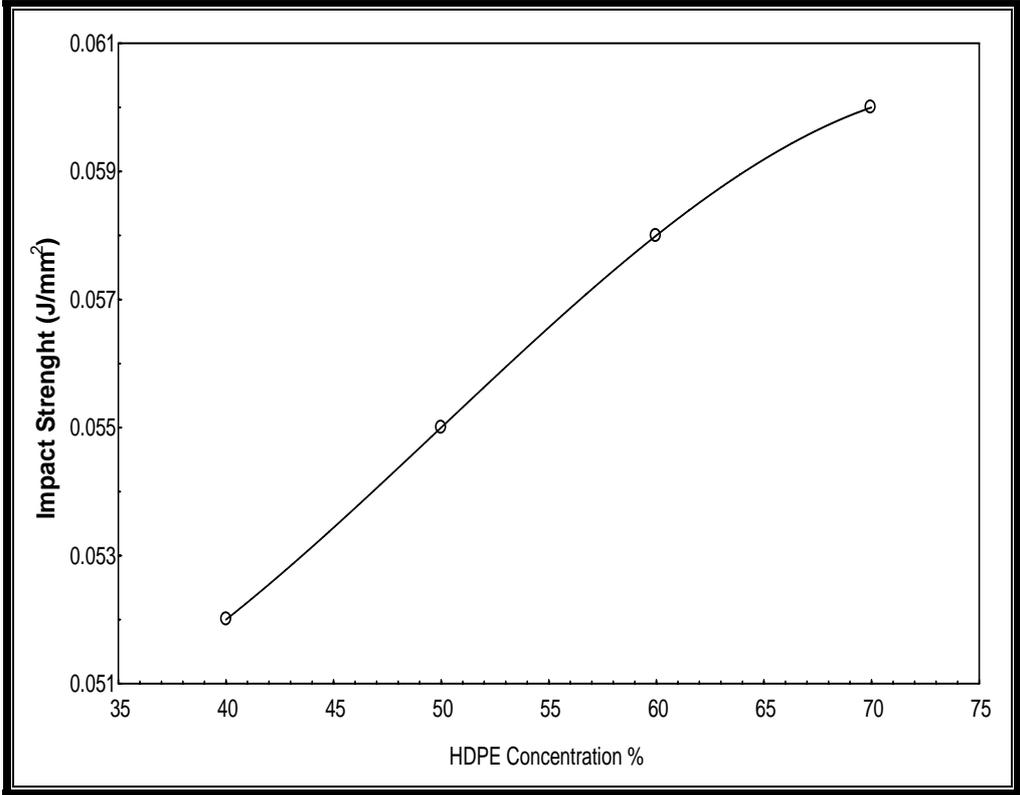
**Figure (3) The Impact strength of HDPE/PP/ABS as a function of %HDPE content**
