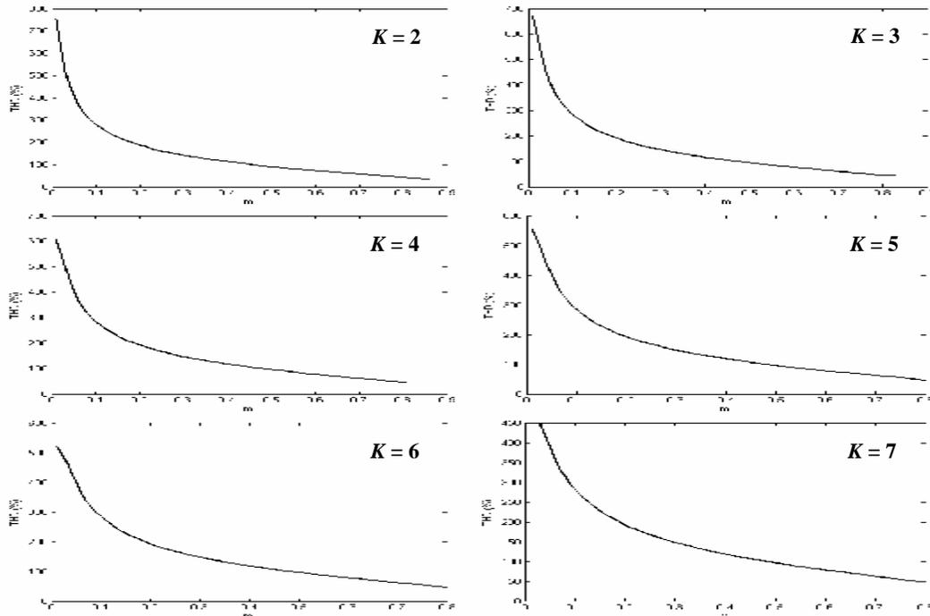
Fig. 5: the Voltage THD vs.  $m$  with different values of  $K$  for Unipolar SHEPWM Inverter
