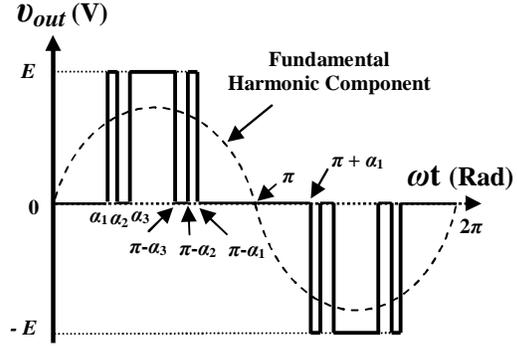
Fig. 2: Unipolar Switching Scheme
