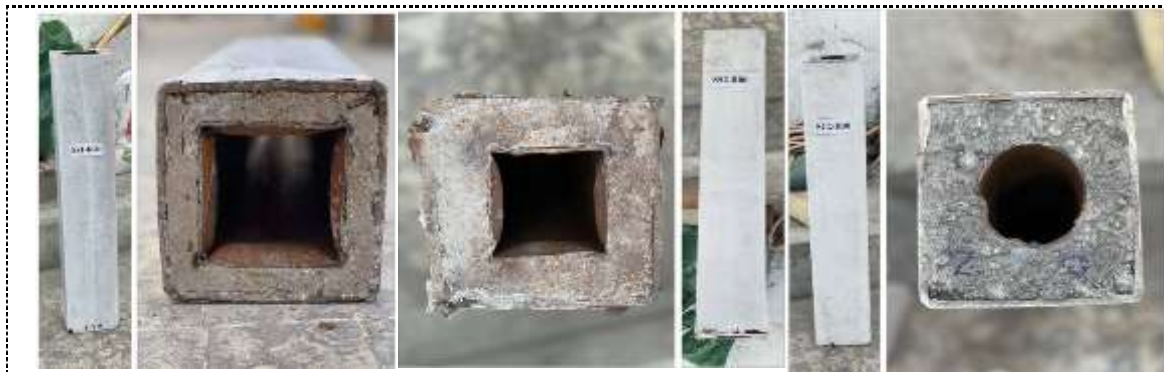
Fig. 13: Failure mechanisms for square-tested columns with axial loading made with 0%RA.
