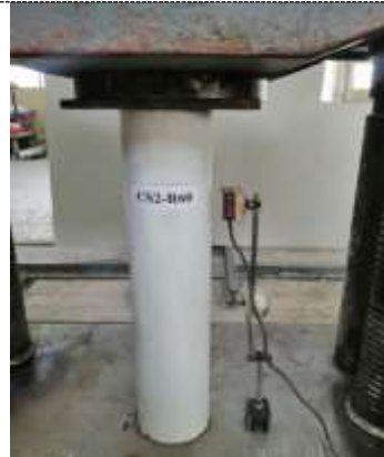
Fig. 10: Installation of the laser LVDT device.
