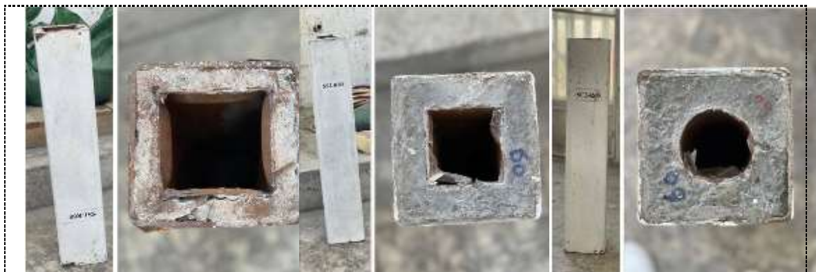
Fig. 17: Failure modes for square-tested columns with axial loading made with 60% RA.
