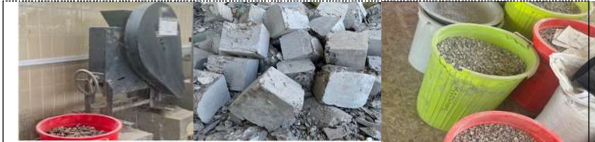
Fig. 3: Recycled aggregate preparation.
