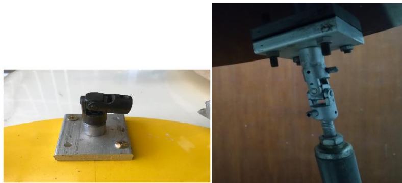
FIG. 4. JOINTS IN UPPER PLATFORM (MOVING PLATFORM) (A) UNIVERSAL JOINT USED IN FIRST MODEL, (B) UNIVERSAL JOINT USED IN SCONED MODEL.
