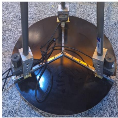
FIG. 1. LOWER PLATFORM WITH THREE RAILS FOR CHANGING DIAMETER.
