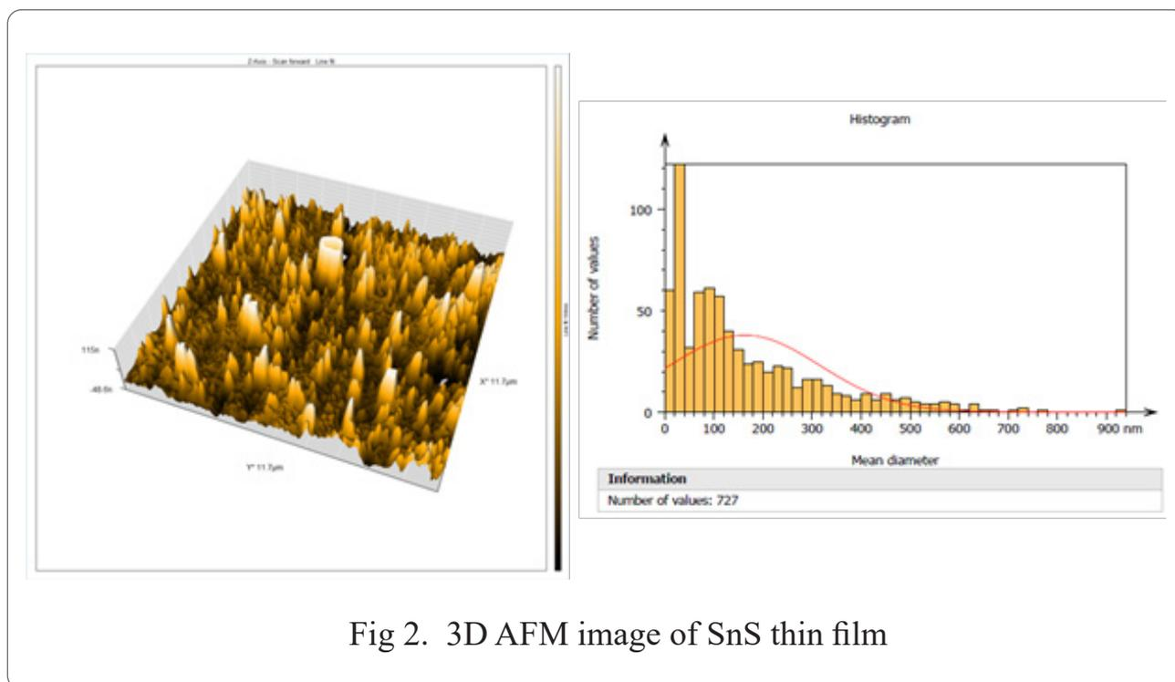
Fig 2. 3D AFM image of SnS thin film
