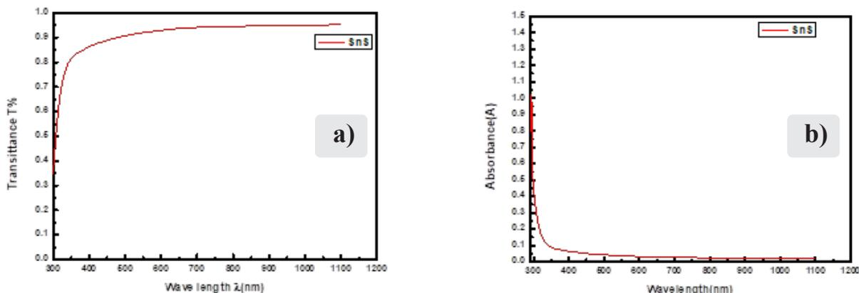
Fig. 3 a) Transmittance and b) Absorbance as a function wavelength of SnS film
