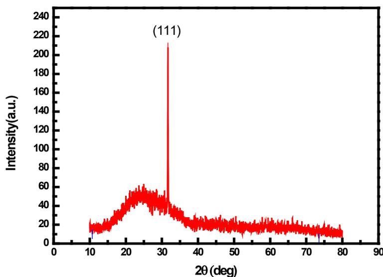
Fig 1. X-ray diffraction pattern of SnS thin film.
