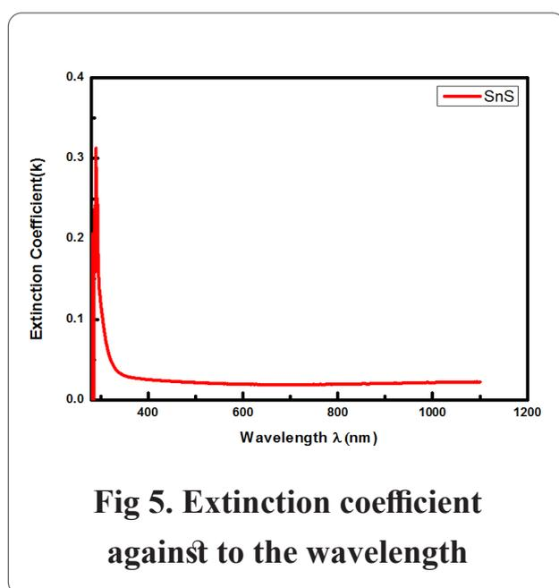
**Fig 5. Extinction coefficient against to the wavelength**
