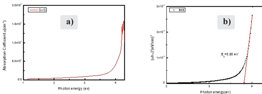
Fig 4. a) Absorption coefficient and b) energy band gap for SnS film.
