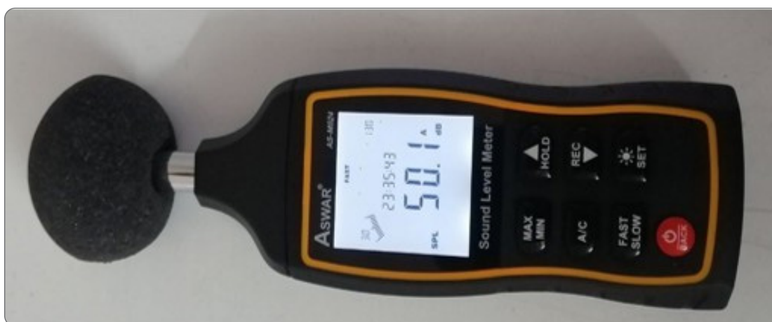
Fig. 2: Sound level meter (AS-M524) used in the present work.
