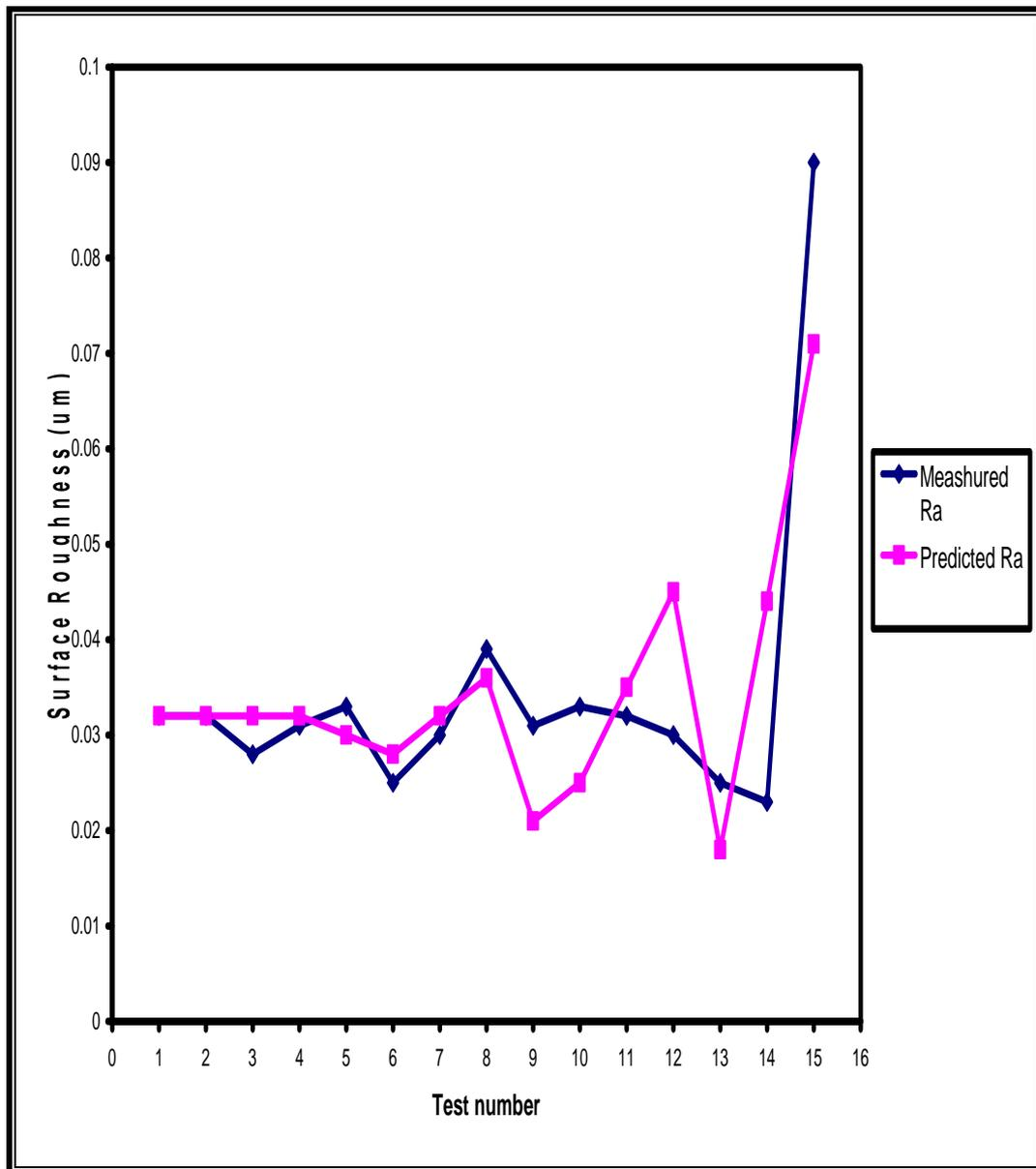
**Figure (2): The diagram of the measured and predicted surface roughness for the experimental data using the commercial statistical package (SPSS)**
