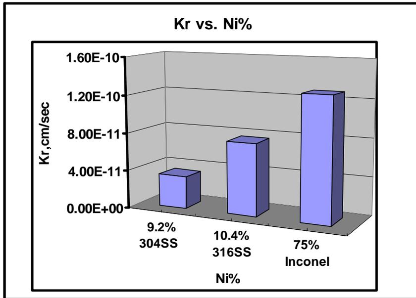
Figure (6) Scale removal rate constant vs. Ni% for different alloys oxidized at 450 °C in LBE.
