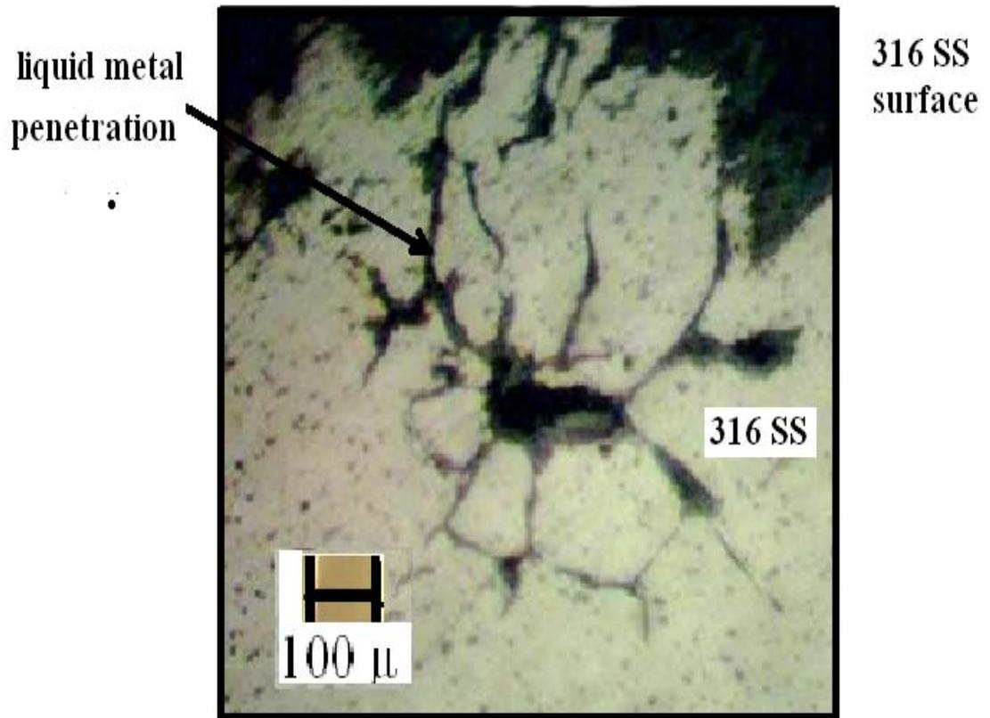
**Figure (8) . Lead-Bismuth penetration in 316SS after 100 hrs
