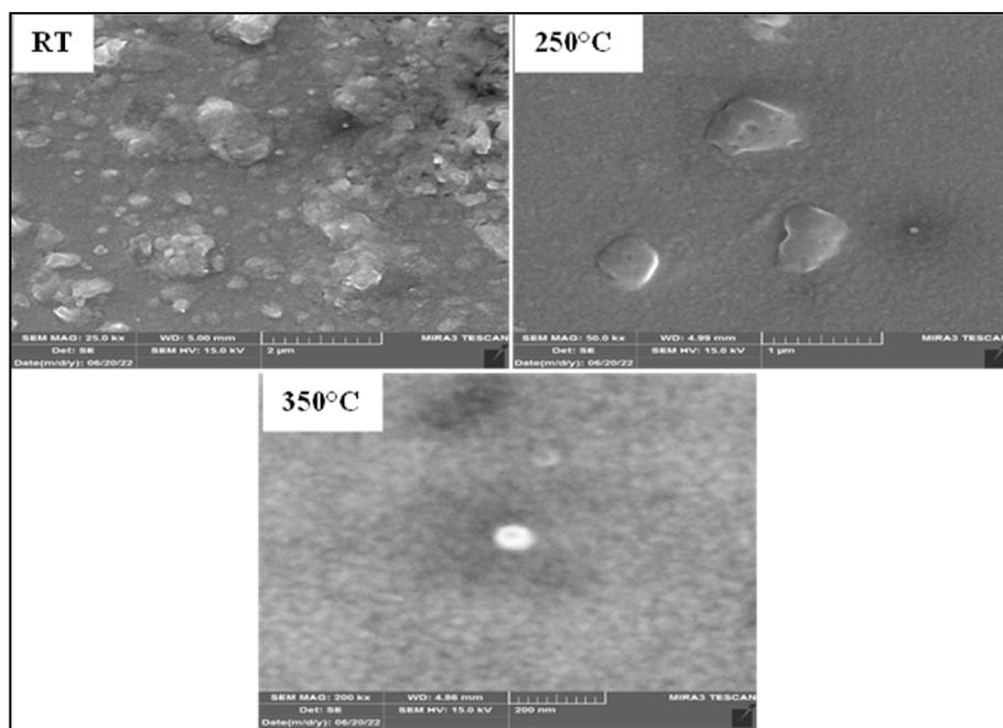
Fig. 5. SEM images of ZnTe thin films before and after annealing at  $x = 7\%$ .
