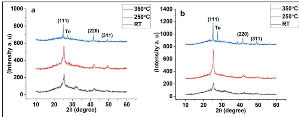
Fig. 2. Pattern X-ray diffraction for (Cd: ZnTe) thin films with two impurity ratios. (a) 5 %. (b) 7 %.
