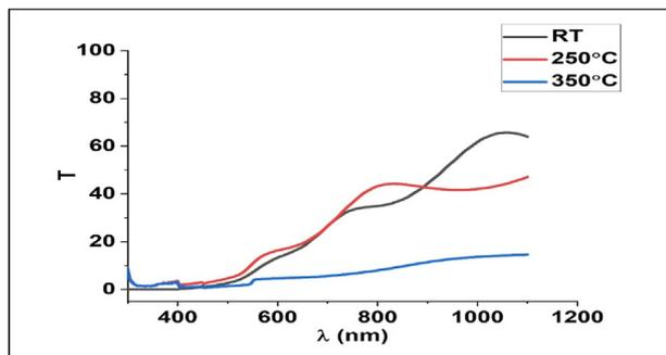
Fig. 6. Transmittance spectra of ZnTe at room temperature and the annealing (250, 350)°C.
