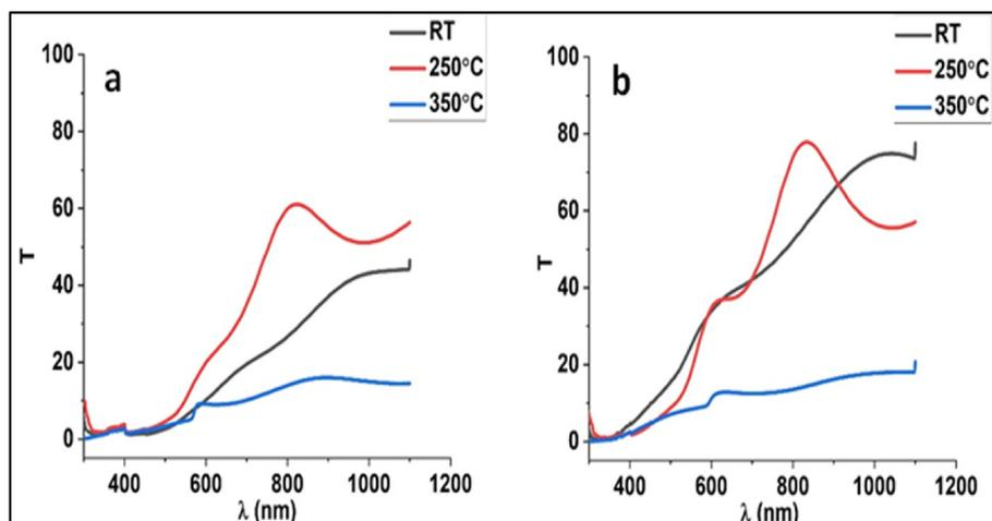
Fig. 7. Transmittance spectra of ZnTe: Cd at room temperature and the annealing temperatures (250, 350)°C, at (a)  $x = 5\%$ , (b)  $x = 7\%$ .
