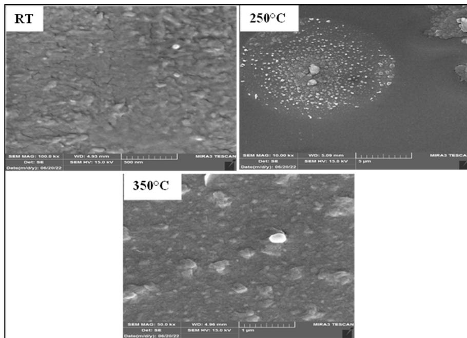
Fig. 4. SEM images of ZnTe thin films before and after annealing at  $x = 5\%$ .
