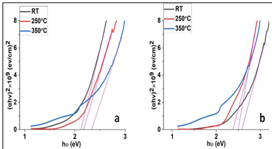
Fig. 9. Energy gap values of ZnTe at room temperature and the annealing (250, 350)°C, at (a)  $x = 5\%$ , (b)  $x = 7\%$ .
