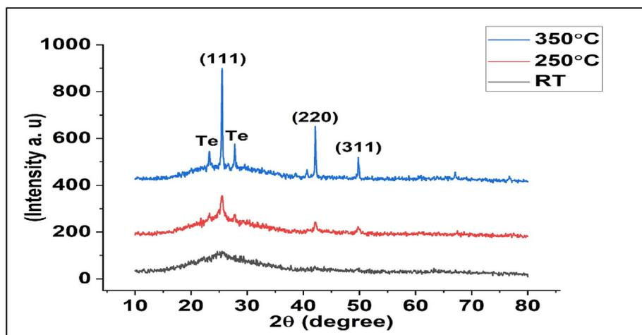
Fig. 1. X-ray diffraction pattern of ZnTe before annealing and after.
