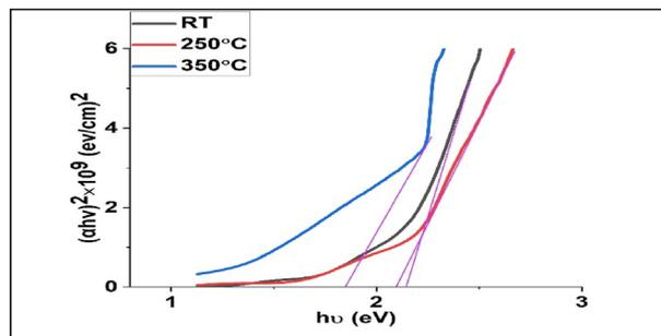
Fig. 8. Energy gap values of ZnTe at room temperature and the annealing (250,350)°C.
