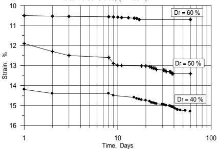
Fig. (11): Effect of relative density on creep for dry samples, (N1 soil).
