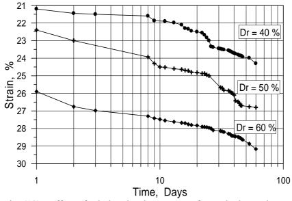
Fig. (12): Effect of relative density on creep for soaked samples, (N1 soil).
