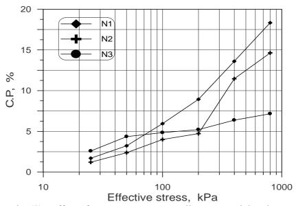
Fig. (8): Effect of gypsum content on collapse potential under different stresses.
