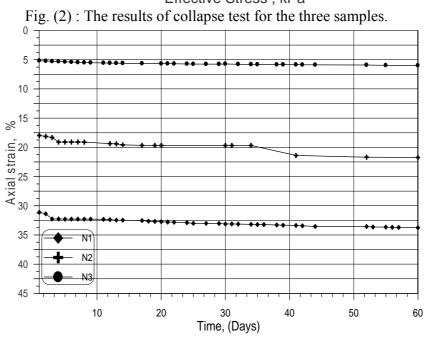
Fig. (3): Variation of strain with time (creep).
