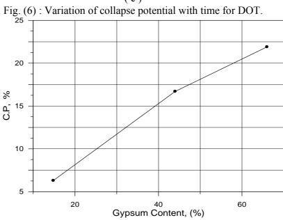
Fig. (7): Effect of gypsym content on long-term collapse potential (under 800 kPa for 60 days).
