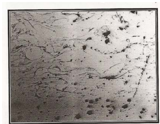
Fig. (12): Optical microscopy picture, (100X), shows the microstructure of the base with the coating layer, unetched.
