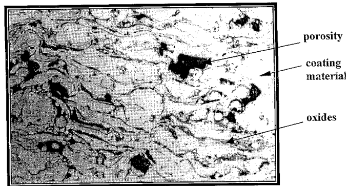
Fig (10): A typical microstructure of a sprayed coating showing the lamellar structure, oxides and porosity, (100X) unetched.
