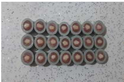
Figure (1): Teeth poured into the acrylic mold with a plastic ring.
