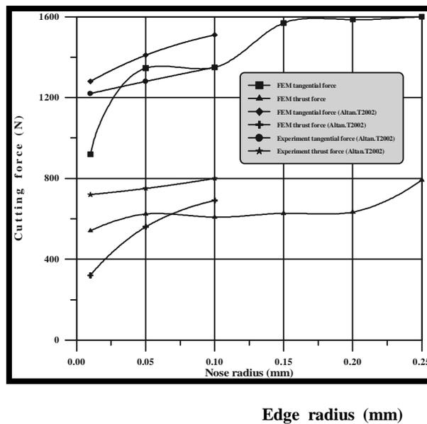
Fig.(6):Comparison of predicted tangential force and thrust force with experimental data Ref.[8].
