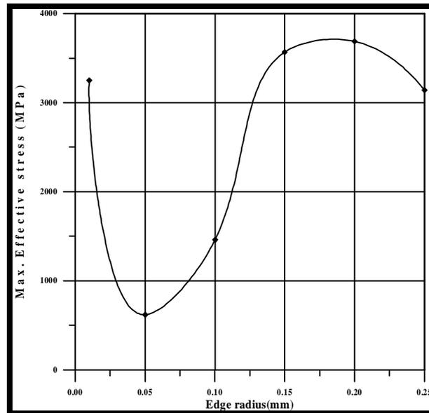
Fig. (5): Relation between edge radius and maximum effective stress.
