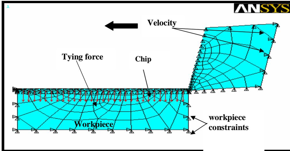
Fig. (1): Representative model boundary conditions (showing the workpiece constraints, tying force between chip and workpiece, velocity direction of the cutting tool).
