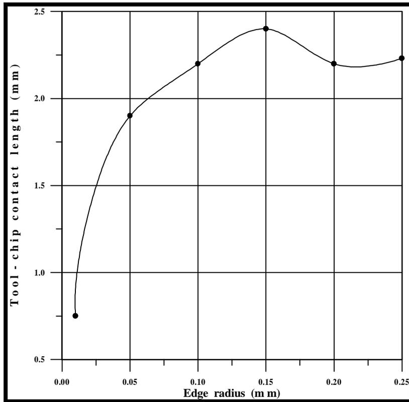
Fig. (7): Effect of edge radius on contact length at tool - chip interface for the simulated tests.
