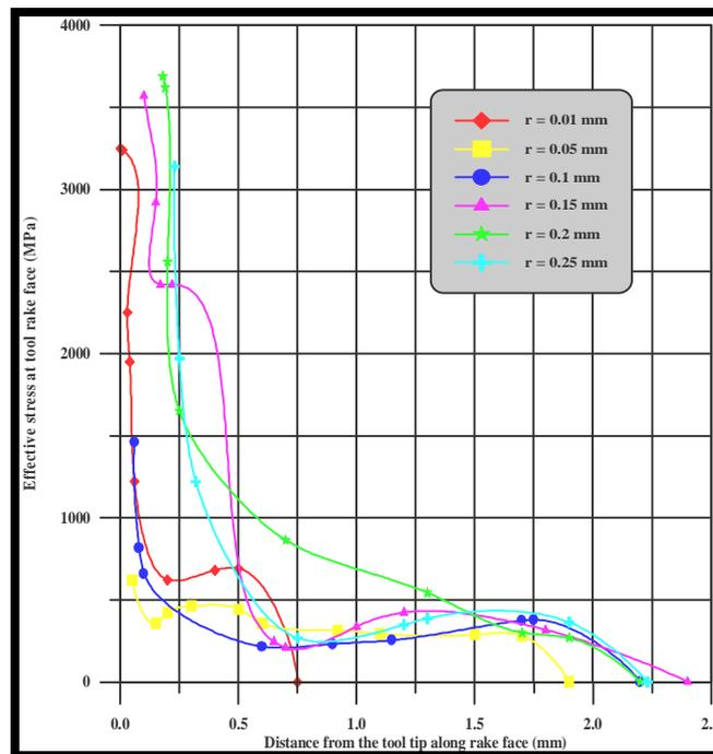
Fig. (4): Predicted effective stress ( $\sigma_n$ ) distributions on the rake face of the honed tool with different edge radii.
