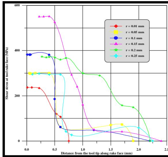
Fig. (3): Predicted shear stress ( $\tau_r$ ) distributions on the rake face of the honed tool with different edge radii.
