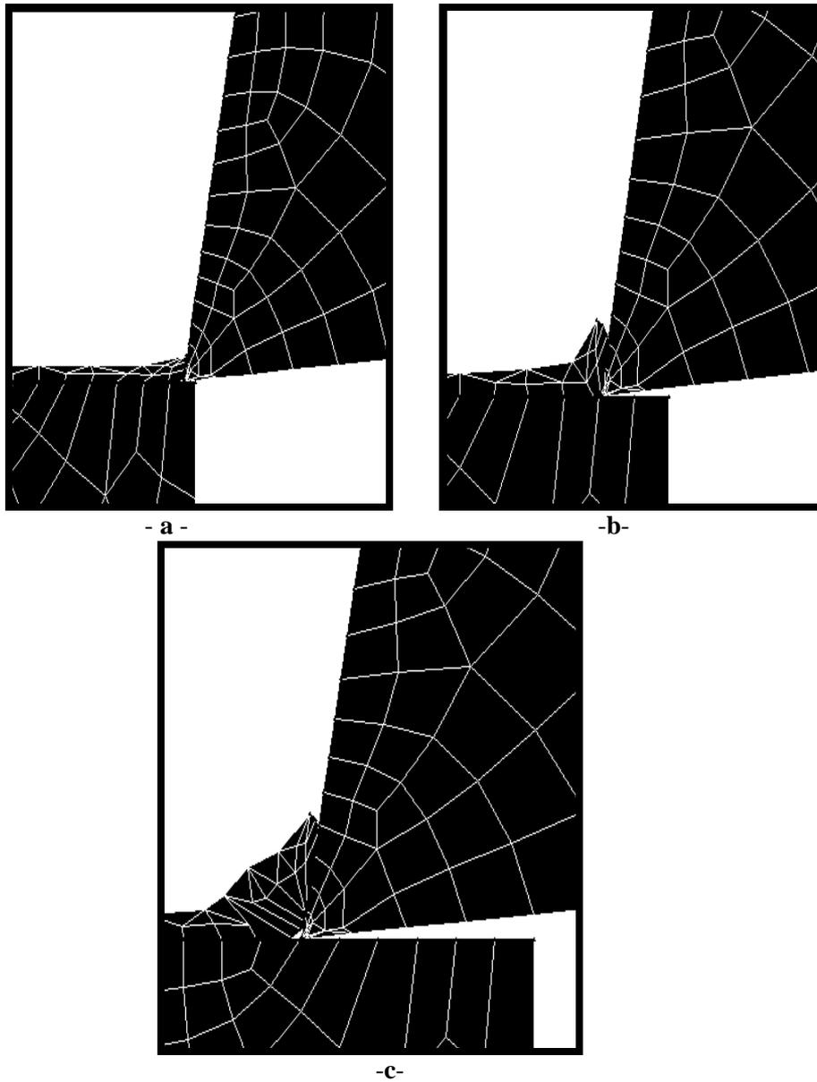
Fig. (2): The stages of the simulation tool advance through the workpiece in steady state condition with different cutting distances:
