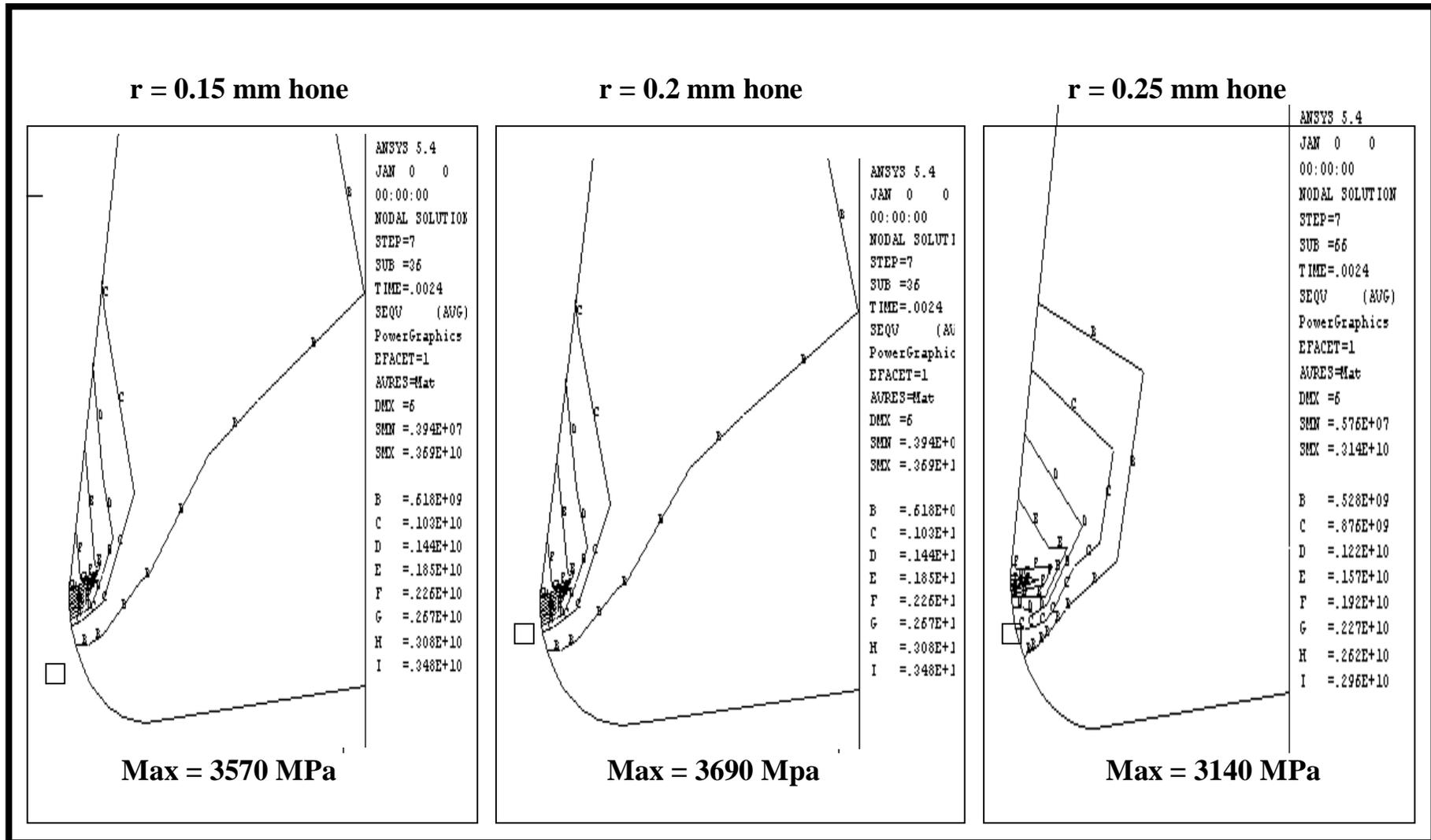
Appendix (B): The effect of edge radius on tool effective stresses (AISI 1006 steel) for the simulated tests.
