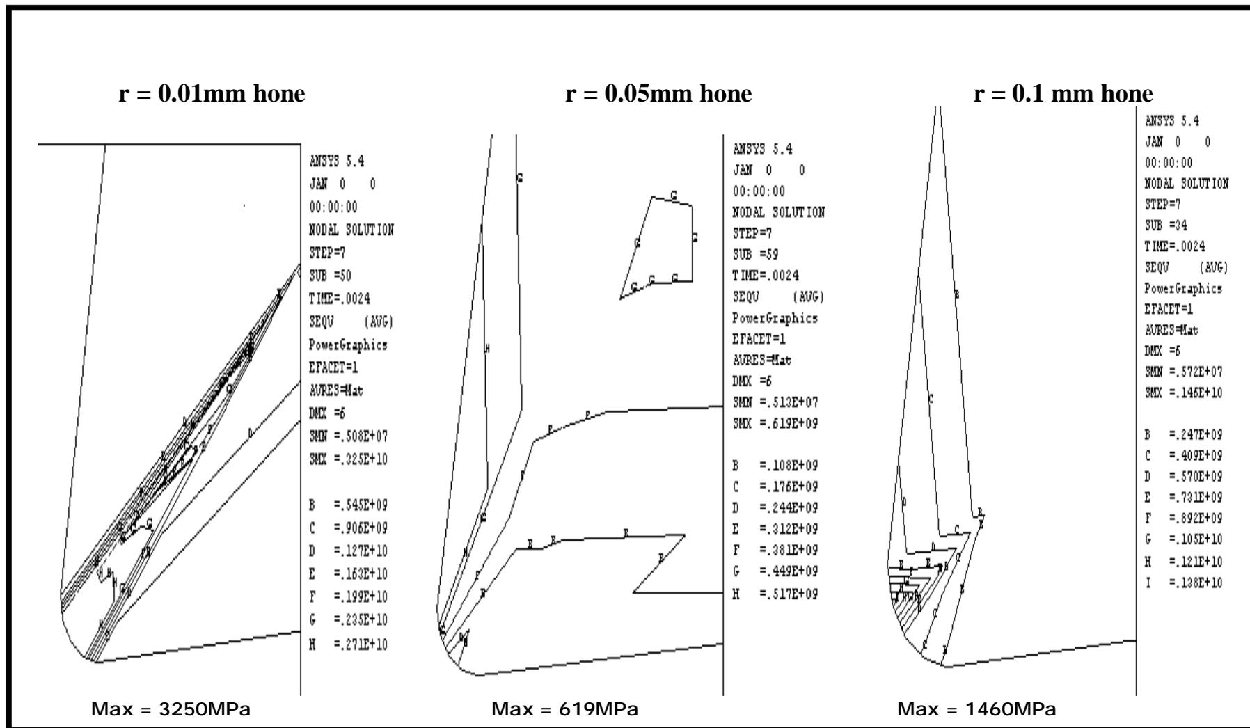
Appendix (A): The effect of edge radius on tool effective stresses (AISI 1006 steel) for the simulated tests.
