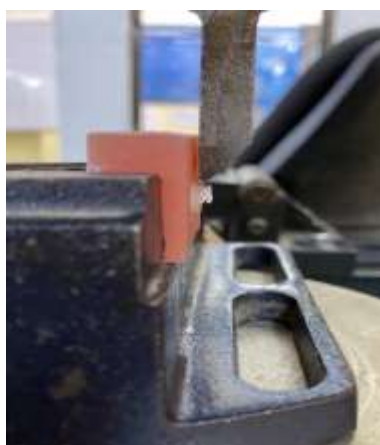
Figure (3): Debonding of the bracket
