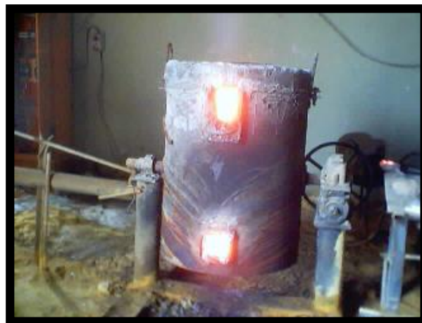
Figure (2) A crucible gas furnace which used in this work
