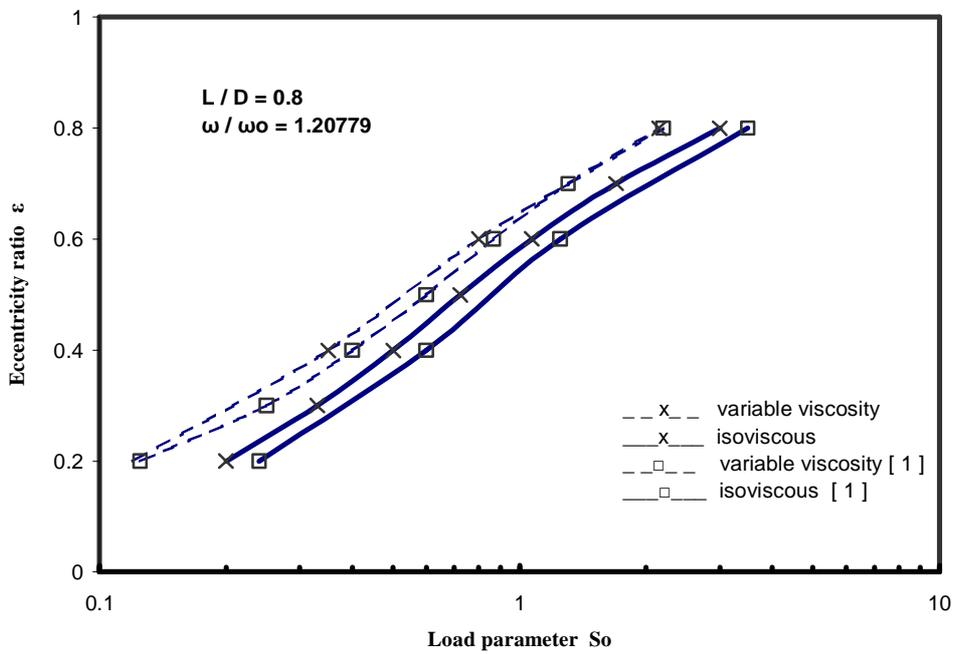
Fig. 4 .Variation of eccentricity ratio with load parameter
