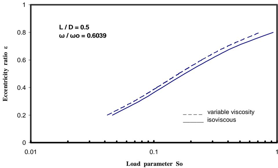
Fig. 5.Variation of eccentricity ratio with load parameter
