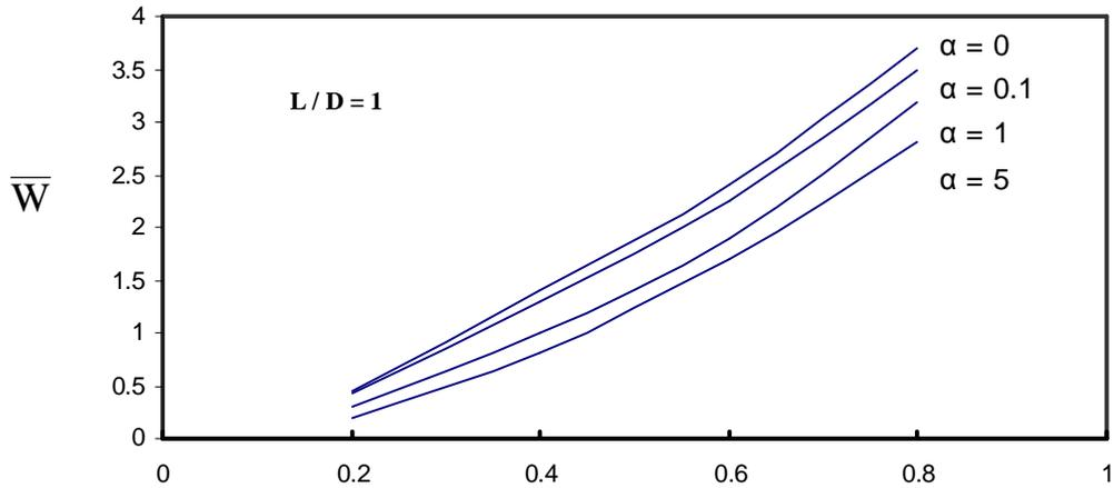
Fig 17 Variation of dimensionless Load capacity with eccentricity ratio . Variable viscosity
