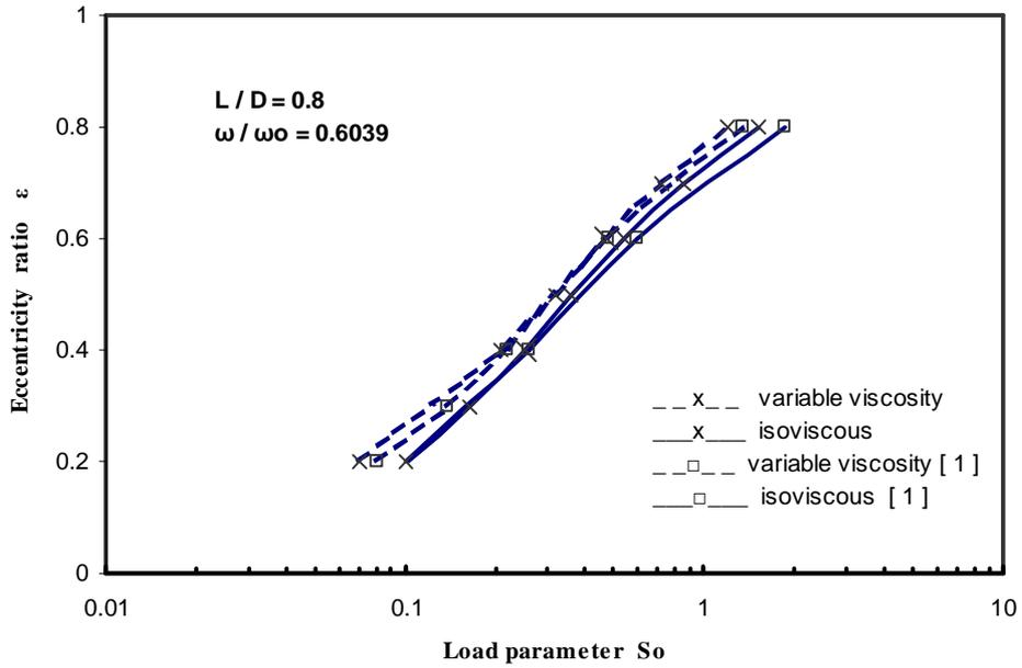
Fig. 3 .Variation of eccentricity ratio with load parameter
