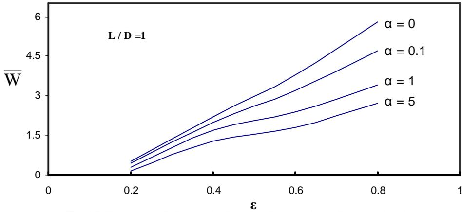
Fig 15 Variation of dimensionless load capacity with eccentricity ratio . isoviscous [ 5 ]
