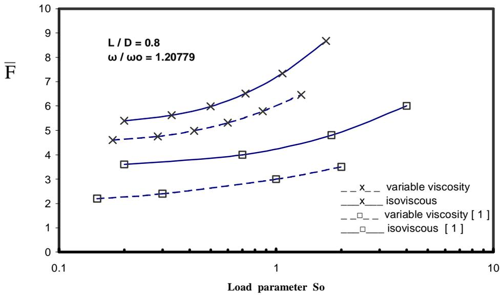
Fig 12 .Variation of dimensionless frictional force with load parameter
