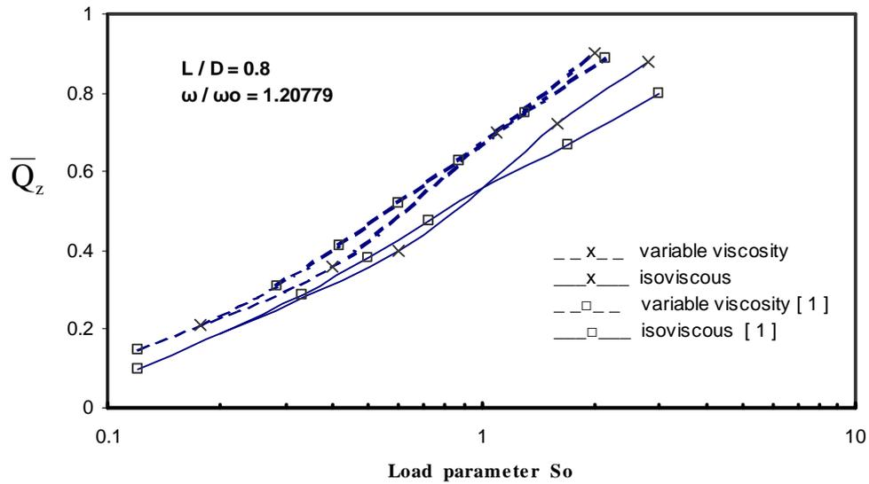
Fig. 8. Variation of dimensionless side flow rate with load parameter
