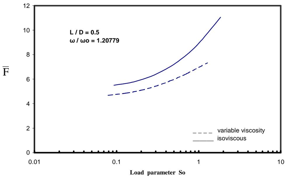
Fig. 14 .Variation of dimensionless frictional force with load parameter
