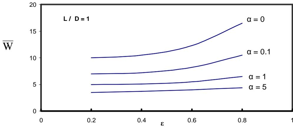
Fig 20 Variation of dimensionless frictional force with eccentricity ratio .isoviscous [ 5 ]
