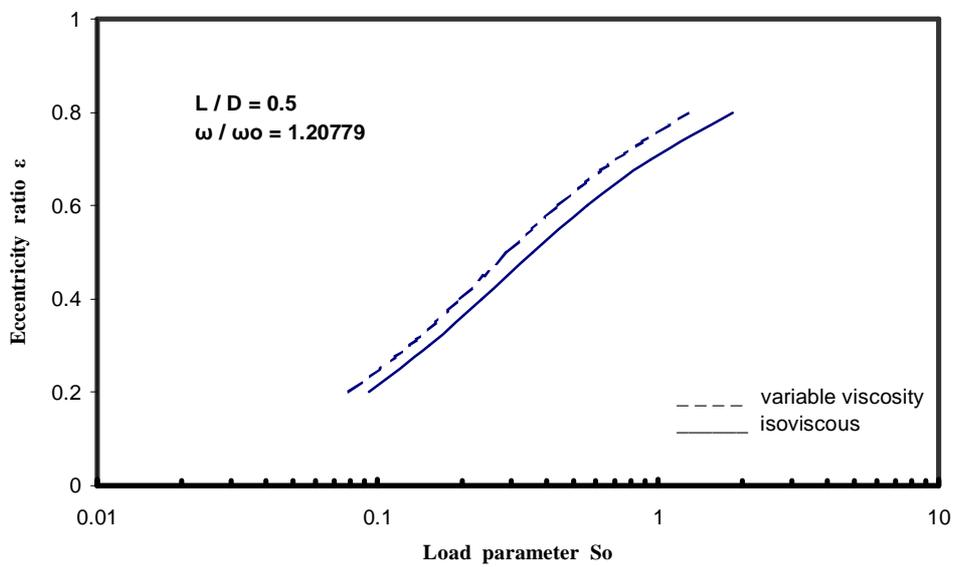
Fig. 6 .Variation of eccentricity ratio with load parameter
