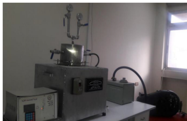
Fig. 3. The gas sensing apparatus.
