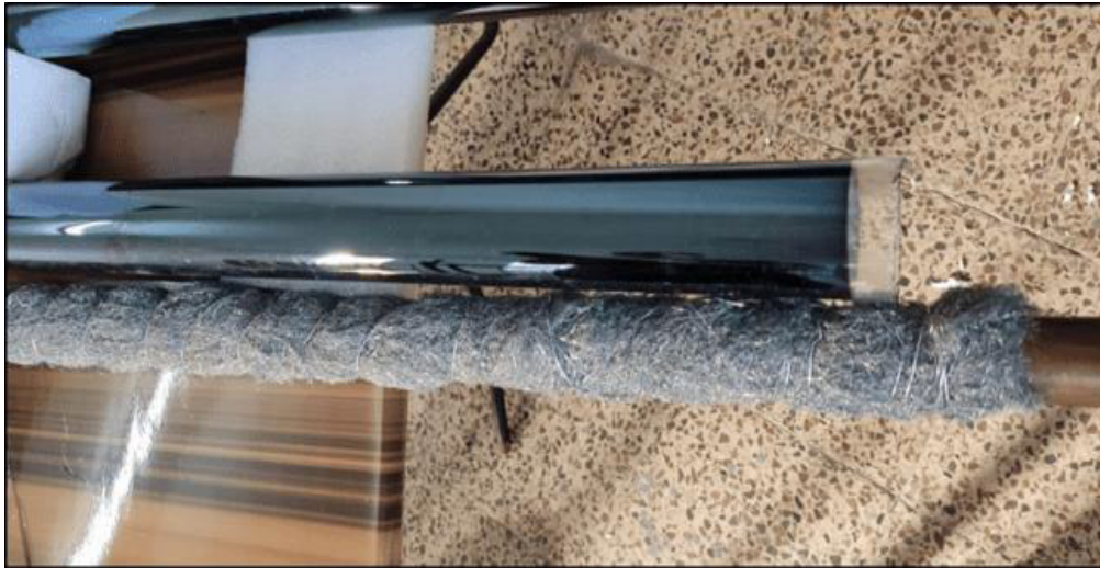
Fig. 3. Primary materials for the copper tube surrounded by aluminum fiber and black chrome-coated glass.
