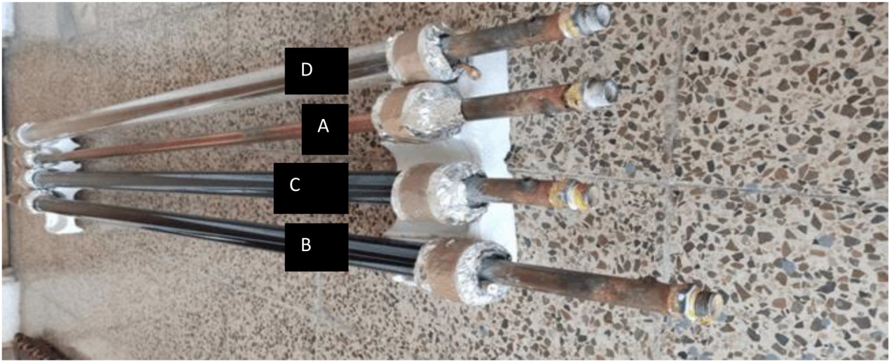
Fig. 5. Types of receivers used in the study. (A) Copper tube surrounded by air. (B) Copper tube surrounded by aluminum fiber, black chrome-coated glass, and vacuum. (C) Copper tube surrounded by phase change material and black chrome-coated glass. (D) Copper tube coated by transparent white vacuum-sealed glass.
