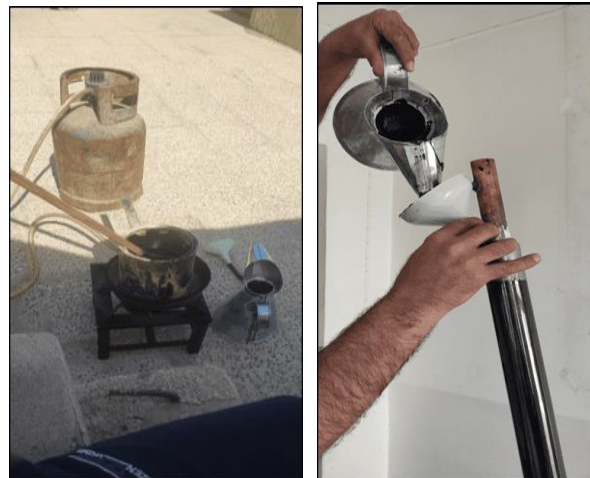
Fig. 4. Primary materials for the copper tube surrounded by phase change material and black chrome-coated glass.
