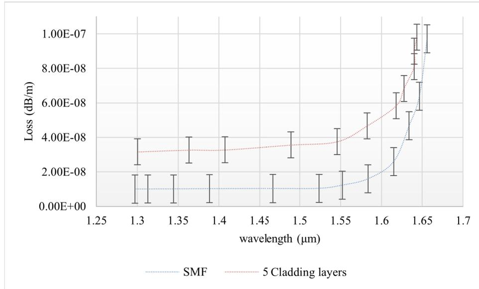
**Fig. 2.** For bending studies, fibers in structures that have single claddings have been compared with five-zoned fibers. The parameters compared included  $\Delta n = 0.016$ , 4.33 mm core diameter,  $\lambda_c = 1.22$  mm, MFD = 5.22 mm, and  $R = 5$  mm.
