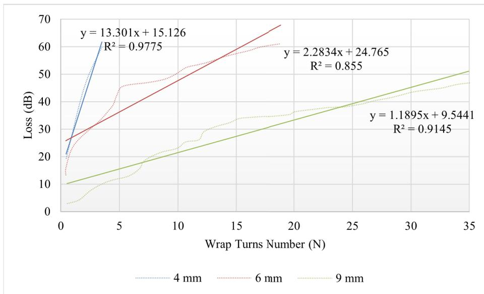
**Fig. 5.** The relationship between the wrap number of turns ( $N$ ) and BL for a range of values from 4 to 8 mm for the radius ( $R$ ).
