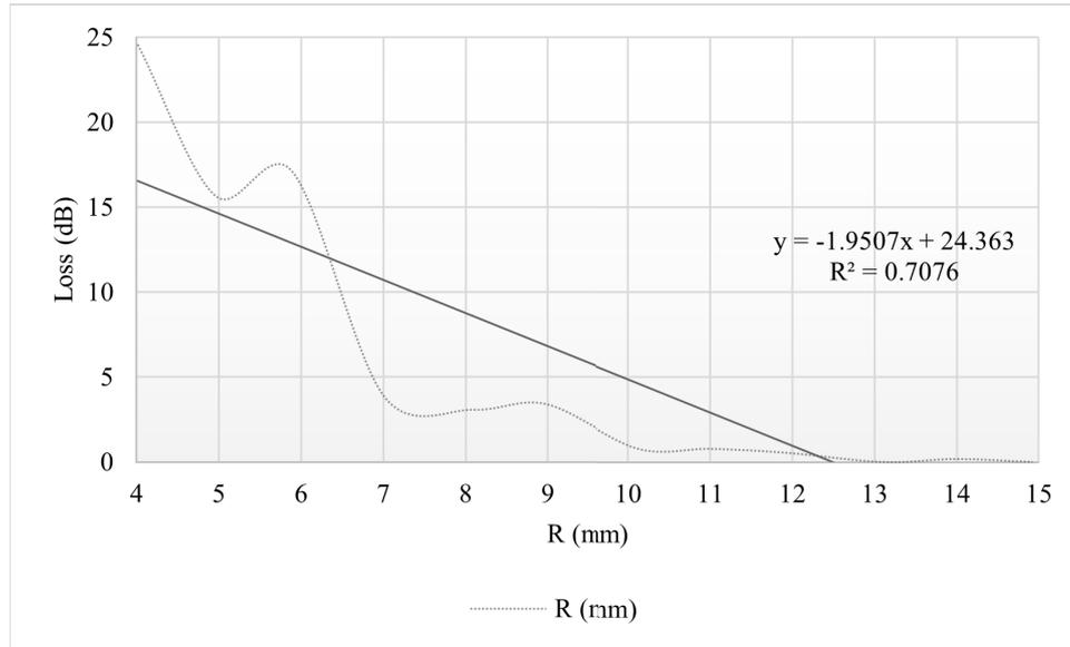
**Fig. 3.** Linear relationship between L and R. The average loss rate decreases per unit increase in radius.
