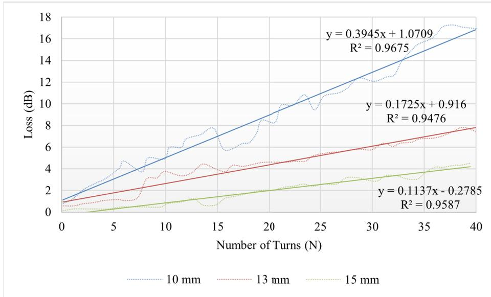
**Fig. 4.** The relationship between  $L$  and  $N$  within the range of 10 to 15 mm for the radius ( $R$ ).  $R^2$  value for all cases close to 1 indicate a strong linearity between  $L$  and  $N$  of each radius.
