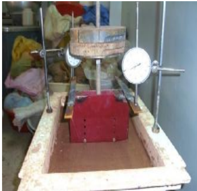
Plate (3) Assembly of loading model of skirt foundation and dial gages .
