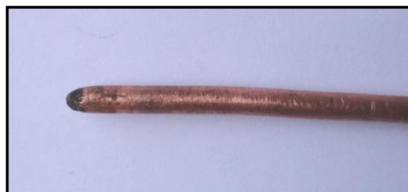
Figure(2-a) Copper electrode before machining .
