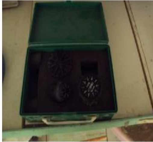
Plate (6) Apparatus of the van shear gauge
