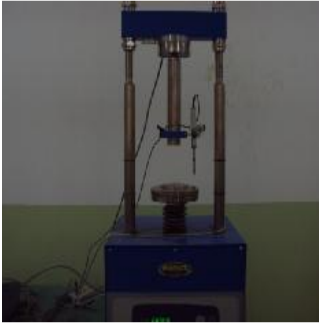
Plate (5) Load cell and indicator
