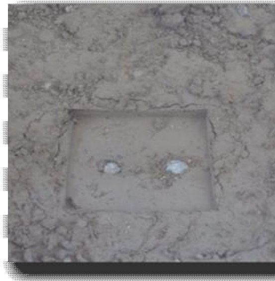
Plate (8) Two piles with raft after test.
