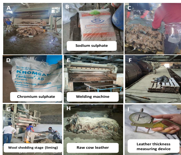
Fig. 1. A look at the stages (A-I) of leather tanning and the chemicals used in tanning factories.
