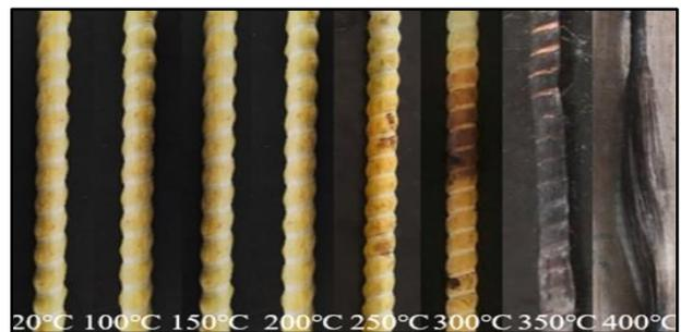
**Figure 3.** GFRP bars after exposure to elevated temperature [26]
