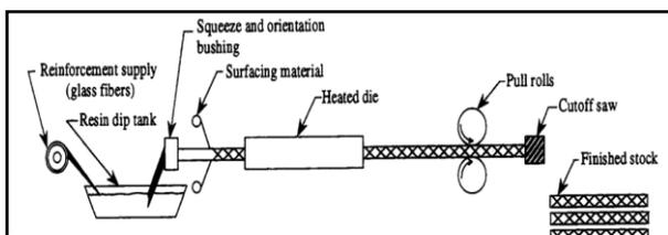
**Figure 2.** Pultrusion of GFRP rebar [20]
