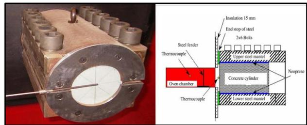
**Figure 9.** Steel mantle with cylinder concrete exposed to oven
