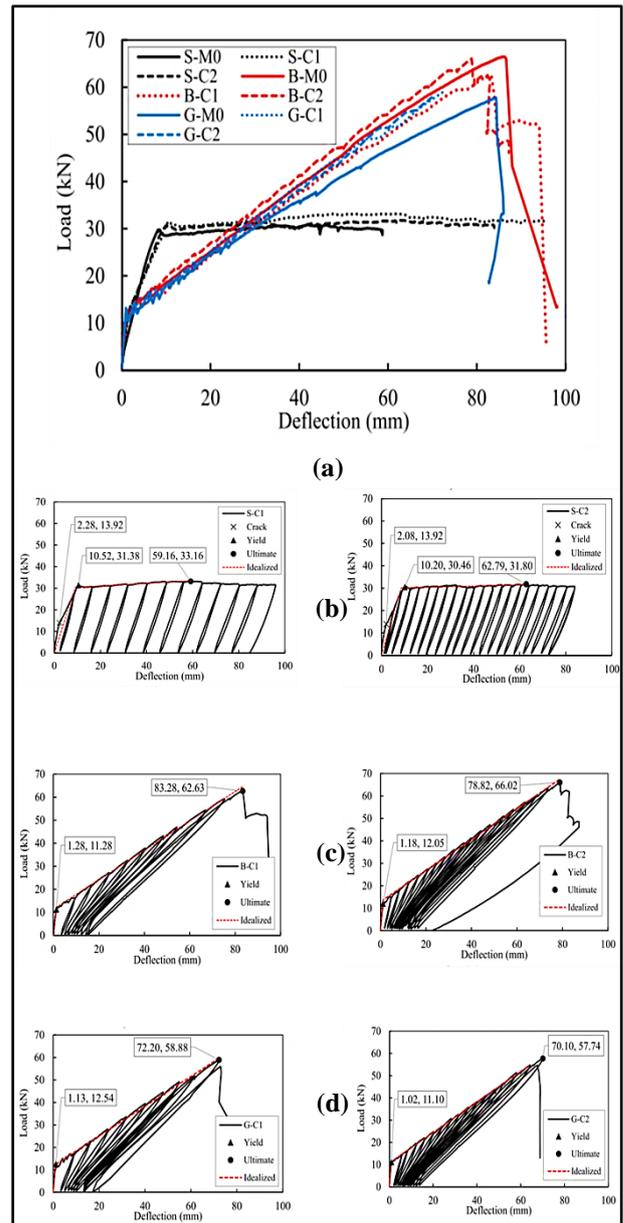
**Figure 15.** Load vs deflection relationships, (a) load vs deflection got monotonic loading, (b) load vs deflection for cyclic load (c1 and c2) of steel reinforcement slabs, (c) load vs deflection for cyclic load (c1 and c2) of BFRP reinforcement slabs, (d) load vs deflection for cyclic load (c1 and c2) of GFRP reinforcement slabs [48]
