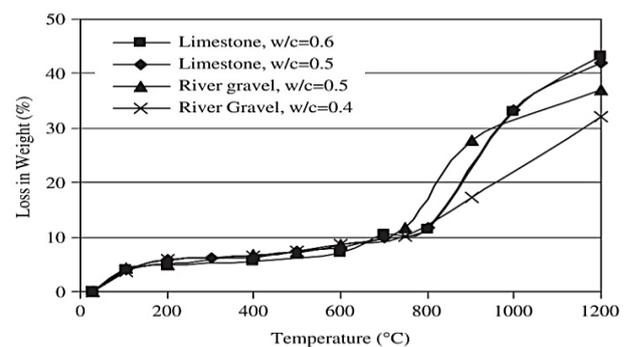
**Figure 7.** Weight reduction of concrete samples exposed to high temperatures [31]
