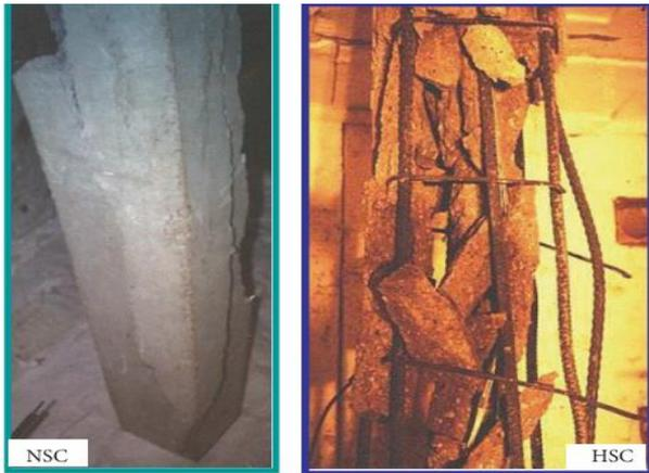
**Figure 11.** Spalling in NSC and HSC columns under fire conditions
