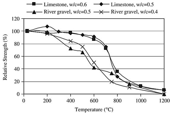
**Figure 8.** Relative strength of concrete mixtures following exposure to high temperatures [31]
