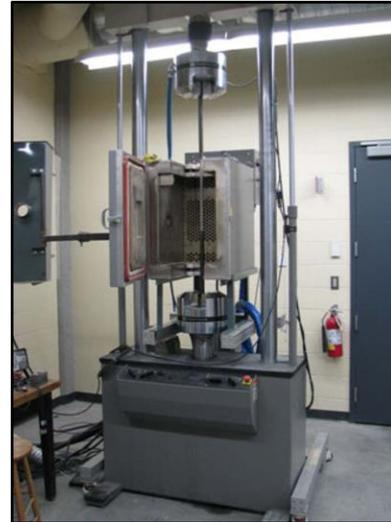
**Figure 5.** Tensile test at the heated chamber [27]
