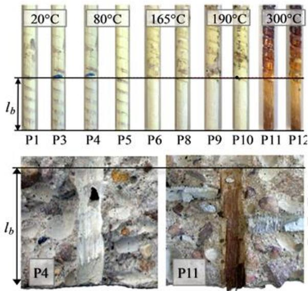
**Figure 6.** Conditioned GFRP bar surface (top) and concrete surface (bottom) following debonding failure [29]
