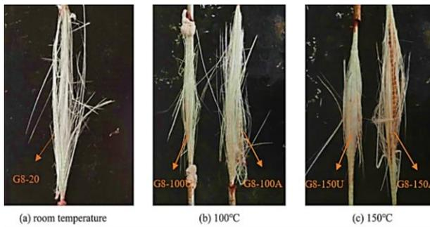
**Figure 4.** Tensile failure mode of specimens under and after high temperatures [26]
