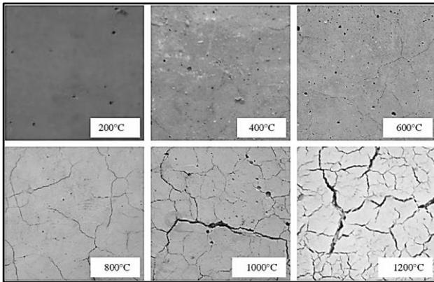
**Figure 10.** Texture of the concrete surface at raised temperatures [31]
