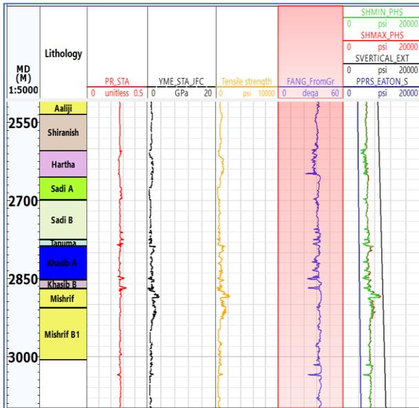
Fig. 4. Static elastic properties, Tensile strength, Friction angle, pore pressure, vertical stress, min and max horizontal stress
