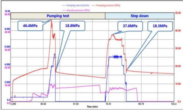
Fig 2. Mini frac test (Syed et al., 2018)
