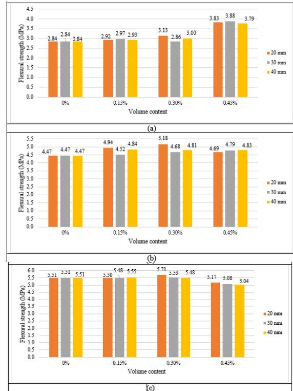
**Fig. 6** Flexural Strength of Concrete Containing Different Volume Contents and Lengths of RFMF at: (a) 3 Days of Curing. (b) 7 Days of Curing. (c) 28 Days of Curing.
