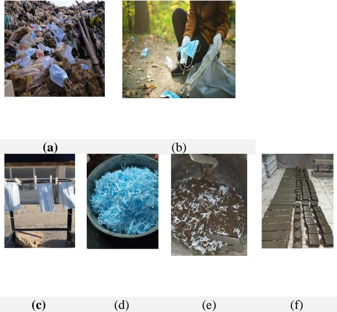
**Fig. 2** The Process Methodology for Incorporating RFMF into Concrete Involved the Following Steps: (a) DFMs at a Landfill. (b) Collection of DFMs. (c) Disinfection of DFMs Using Sunlight. (d) Cutting up the RFMs To Obtain RFMF. (e) Mixing the RFMFs With Concrete in a Mixer. (f) Casting the RFMF Concrete into Molds.
