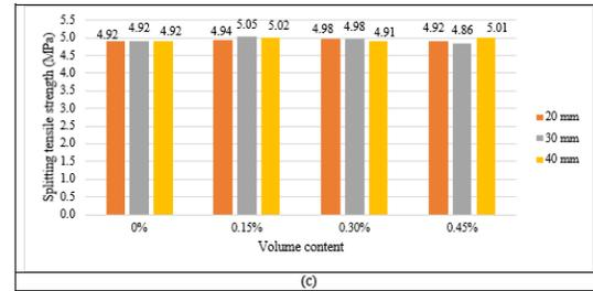
Fig. 5 Splitting Tensile Strength of Concrete Containing Different Volume Contents and Lengths of RFMF at: (a) 3 Days of Curing. (b) 7 Days of Curing. (c) 28 Days of Curing.
