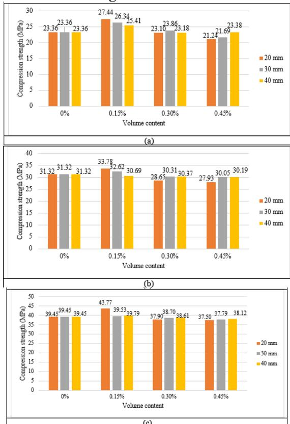
**Fig. 2** Compressive Strength of Concrete Containing Different Volume Contents and Lengths of RFMF at: (a) 3 Days of Curing. (b) 7 Days of Curing. (c) 28 Days of Curing.
