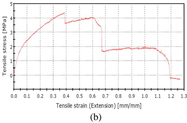
**Fig. 1** Tensile Strength Test of RFMF: (a) The RFMF is Subjected to a Tensile Strength Test. (b) Tensile Stress-Strain Diagram of the RFMF.
