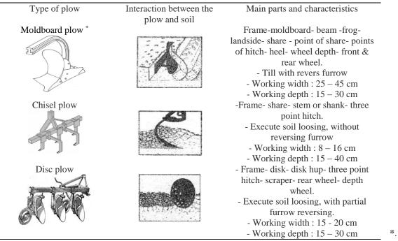
Reversible moldboard plow is consist of the same parts and does the same work, except that it is double
