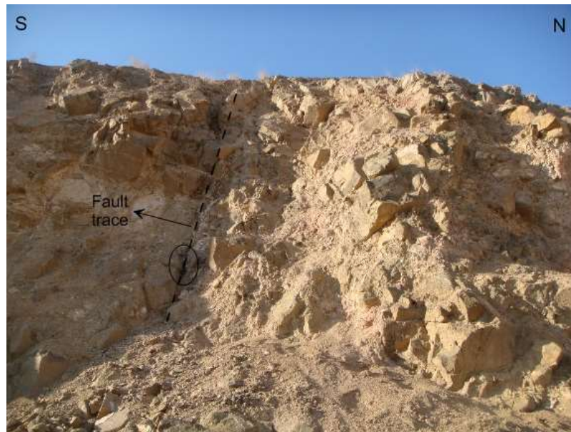
Fig. 10. Sinistral strike-slip fault cutting the basalt, the attitude of this fault is 146^{\circ}/86^{\circ}\text{SW} .
